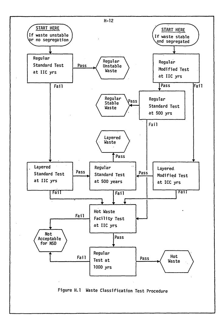
the waste stability index (I8) and the segregation index (IS). In both of " these cases, a waste stream that passes either of the layered tests is tested again in a regular standard waste test at 500 years before being classified as layered waste. - · · · ·
