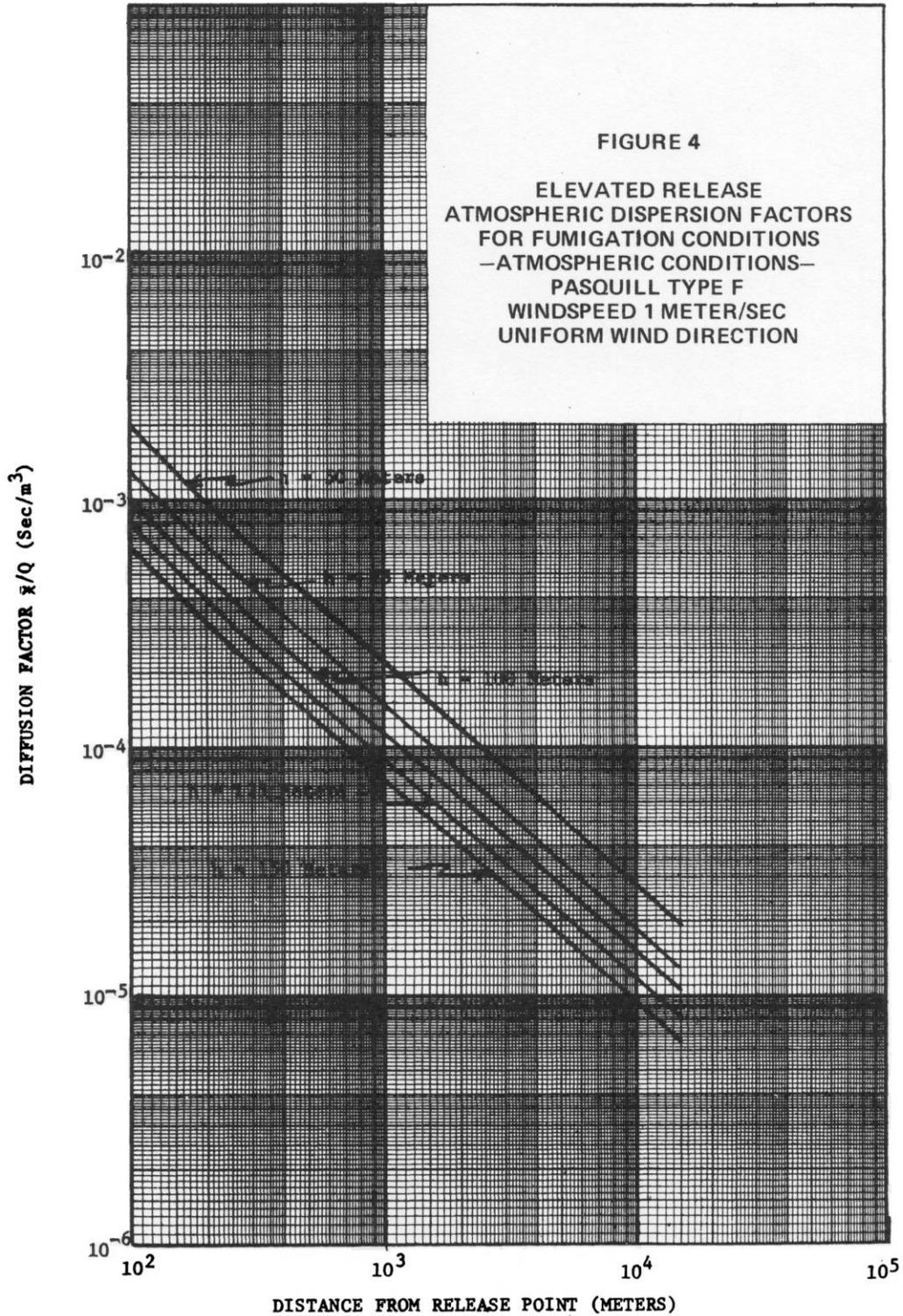
**Figure 4. Elevated Release Atmospheric Dispersion Factors for Fumigation Conditions**
