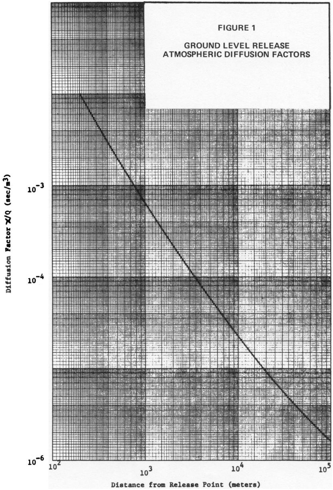
**Figure 1. Ground Level Release Atmospheric Diffusion Factors**
