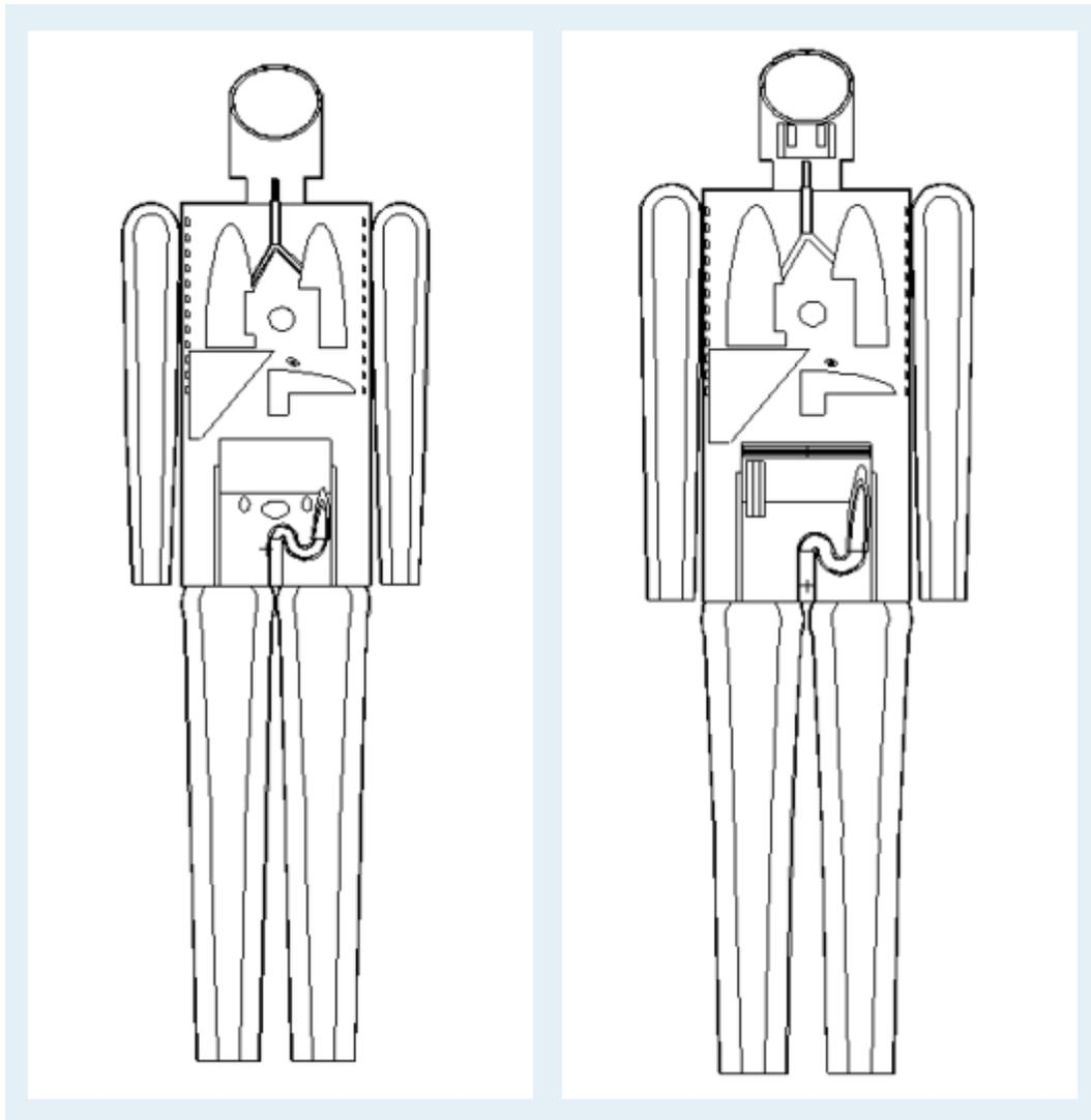
**Figure 7-1 Human Female (left) and Human Male (right) Phantom.**
