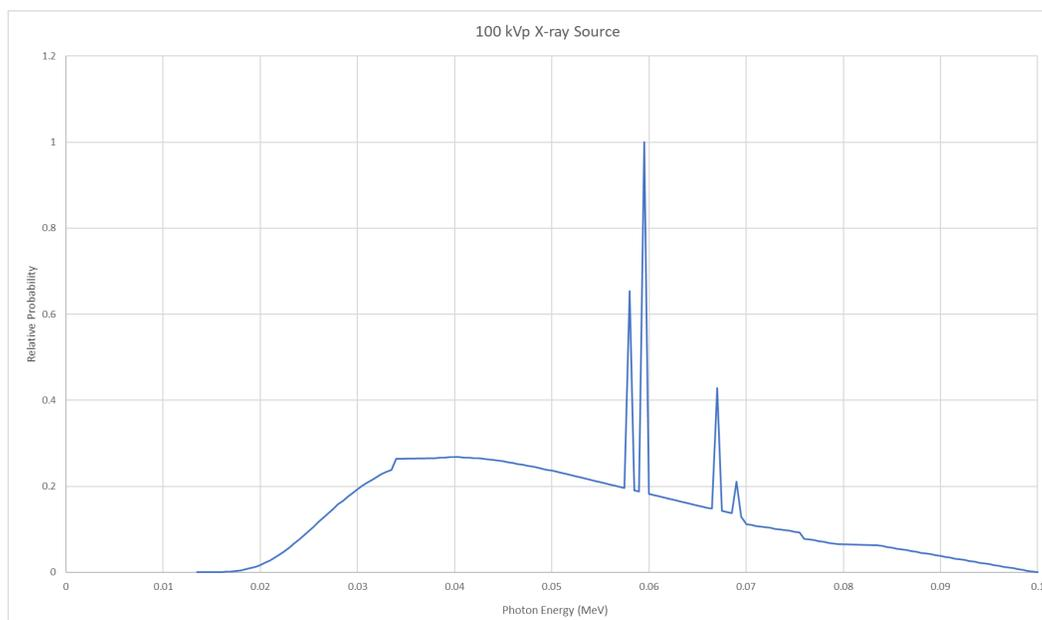
**Figure 6-6 X-ray Energy Spectrum from a Tungsten Target Operated at 100 kVp.**
