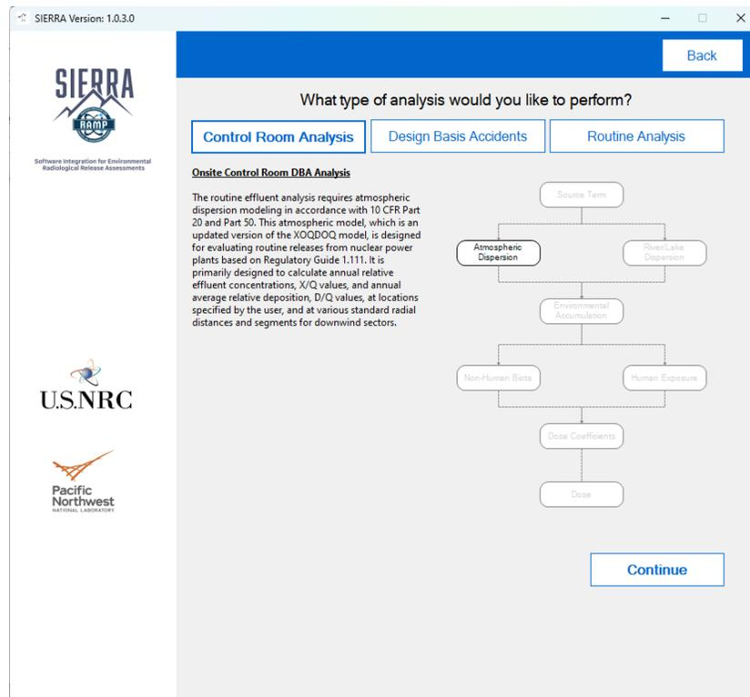
Figure 2-4. SIERRA Analysis Type Selection Panel.
