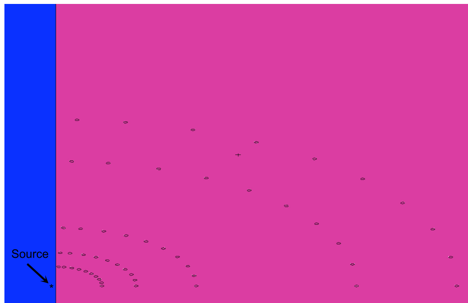
Figure 3-10.: Schematic of the geometry used in MCNP5 to determine the scatter correction factor ( s_c ). Blue is used to represent air and fuchsia is tissue. Note: the source point has been highlighted to orient the simulation.
