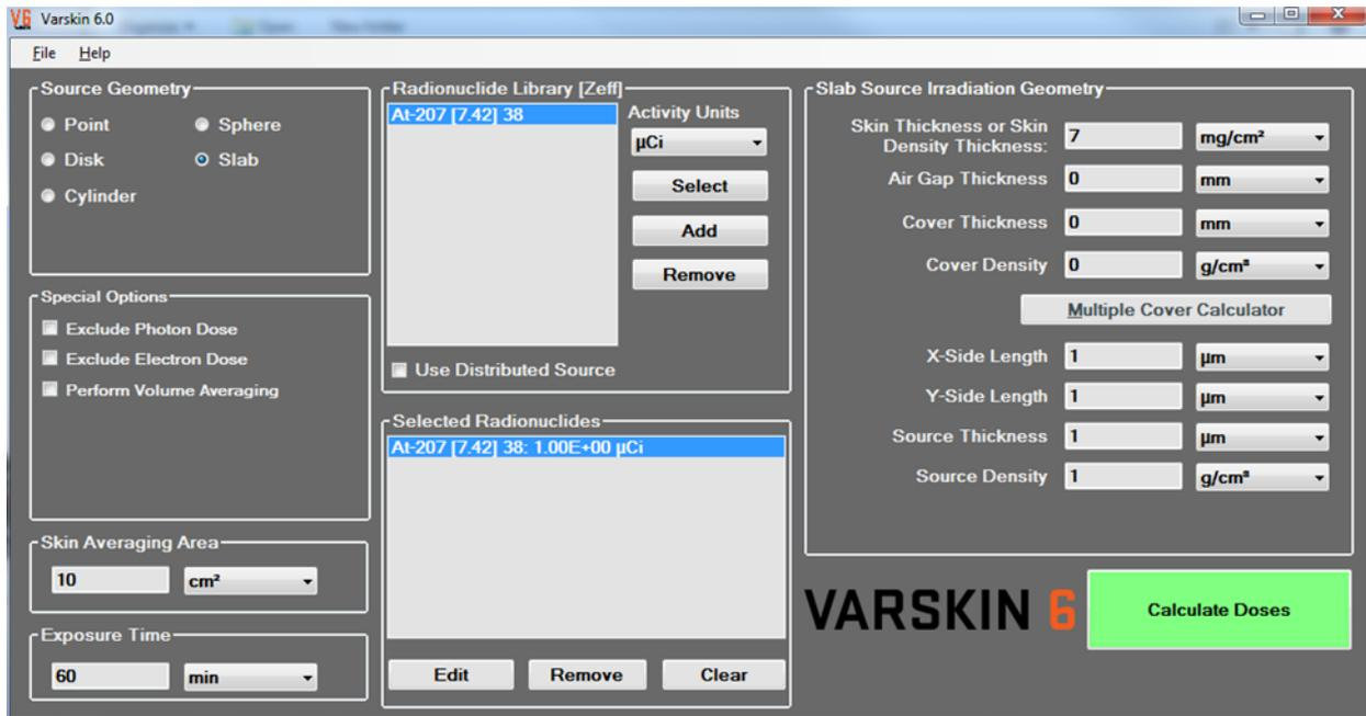
Figure 2-5 Slab Source Geometry Parameters (middle right)
