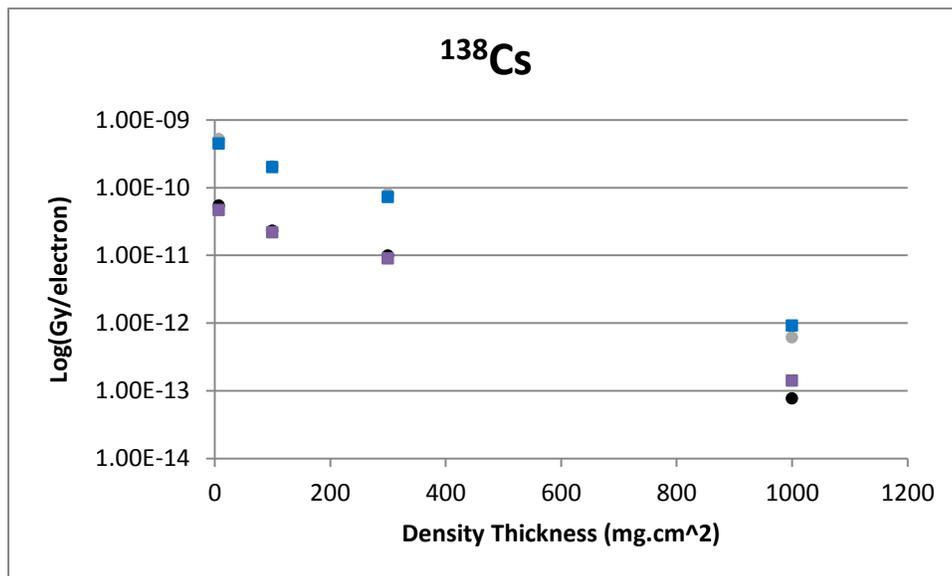
**Figure B-32** A 5 mm Diameter Disk Geometry Comparison of VARSKIN 5 (boxes) and VARSKIN 4 (circles) Predicted Dose Per Initial Beta From  $^{138}\text{Cs}$  as a Function of Density Thickness In Tissue and a Tissue Volume Cylinder of Area 1 cm<sup>2</sup> (upper) and 10 cm<sup>2</sup> (lower), With a Thickness of 20 mm
