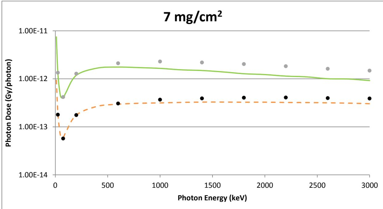
**Figure A-13** A Slab Source Geometry Comparison of VARSKIN 5 (circles) and MCNP5 (lines) Predicted Dose Per Initial Photon as a Function of Photon Energy in Tissue at a Density Thickness of 7 mg/cm<sup>2</sup> and a Tissue Volume Cylinder of Area 1 cm<sup>2</sup> (solid line) and 10 cm<sup>2</sup> (dashed line), With a Thickness of 20 mm
