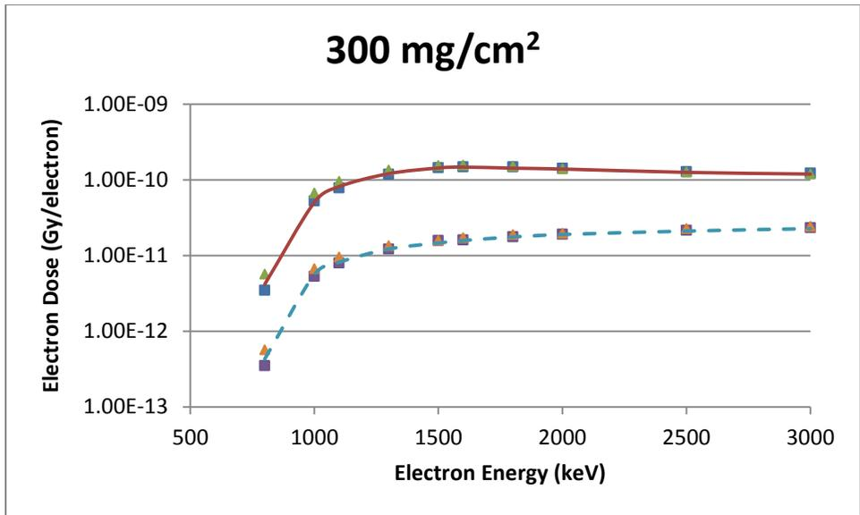
**Figure B-11** A 0.5 mm Diameter Disk Source Geometry Comparison of VARSKIN 5 (boxes), MCNP5 (triangles) and EGSnrc (lines) Predicted Dose Per Initial Electron as a Function of Electron Energy in Tissue at a Density Thickness of 300 mg/cm<sup>2</sup> and a Tissue Volume Cylinder of Area 1 cm<sup>2</sup> (solid line) and 10 cm<sup>2</sup> (dashed line), With a Thickness of 20 mm
