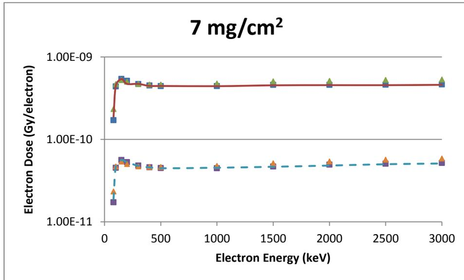
Figure B-17 A 1 mm Diameter Disk Source Geometry Comparison of VARSKIN 5 (boxes), MCNP5 (triangles) and EGSnrc (lines) Predicted Dose Per Initial Electron as a Function of Electron Energy in Tissue at a Density Thickness of 7 mg/cm<sup>2</sup> and a Tissue Volume Cylinder of Area 1 cm<sup>2</sup> (solid line) and 10 cm<sup>2</sup> (dashed line), With a Thickness of 20 mm
