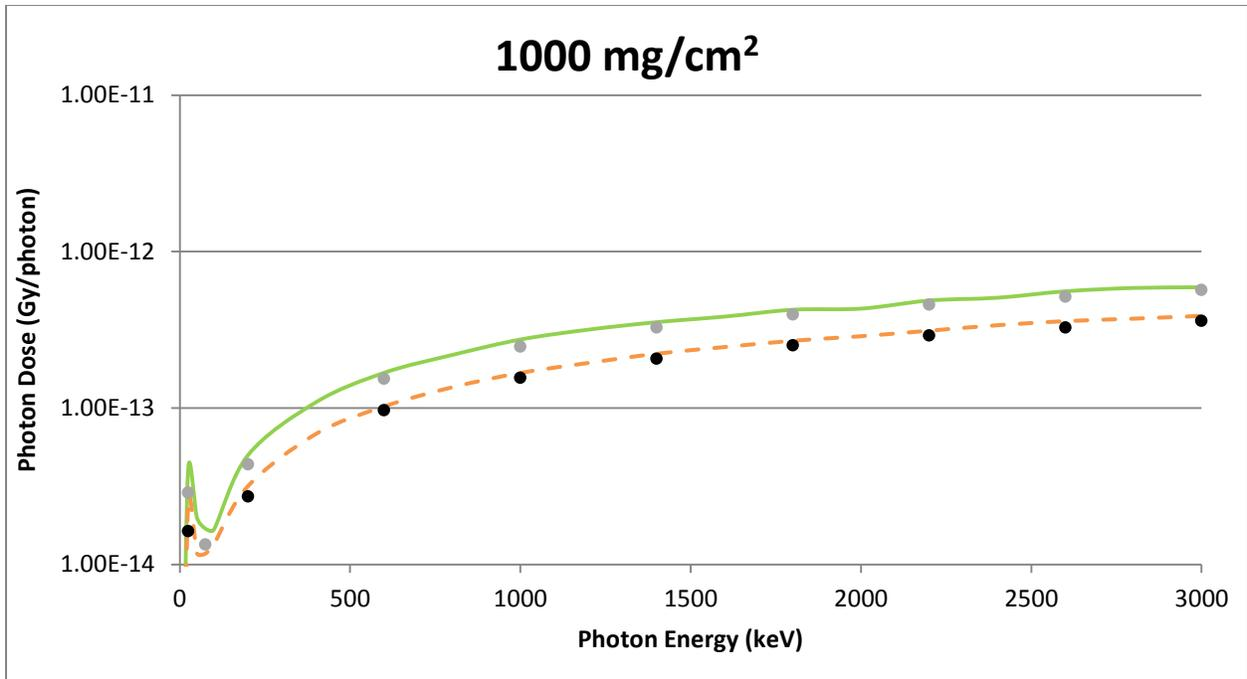
**Figure A-8** A Disk Source Geometry Comparison of VARSKIN 5 (circles) and MCNP5 (lines) Predicted Dose Per Initial Photon as a Function of Photon Energy in Tissue at a Density Thickness of 1000 mg/cm<sup>2</sup> and a Tissue Volume Cylinder of Area 1 cm<sup>2</sup> (solid line) and 10 cm<sup>2</sup> (dashed line), With a Thickness of 20 mm
