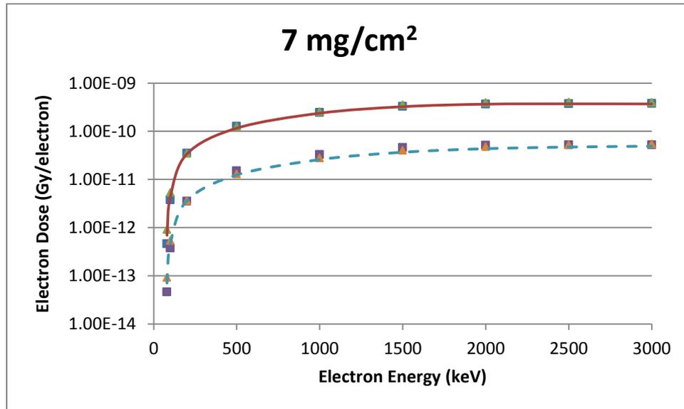
Figure B-33 A Cylindrical Source Geometry Comparison of VARSKIN 5 (boxes), MCNP5 (triangles) and EGSnrc (lines) Predicted Dose Per Initial Electron as a Function of Electron Energy in Tissue at a Density Thickness of 7 mg/cm<sup>2</sup> and a Tissue Volume Cylinder of Area 1 cm<sup>2</sup> (solid line) and 10 cm<sup>2</sup> (dashed line), With a Thickness of 20 mm
