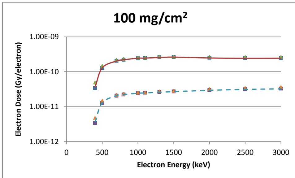
Figure B-18 A 1 mm Diameter Disk Source Geometry Comparison of VARSKIN 5 (boxes), MCNP5 (triangles) and EGSnrc (lines) Predicted Dose Per Initial Electron as a Function of Electron Energy in Tissue at a Density Thickness of 100 mg/cm<sup>2</sup> and a Tissue Volume Cylinder of Area 1 cm<sup>2</sup> (solid line) and 10 cm<sup>2</sup> (dashed line), With a Thickness of 20 mm
