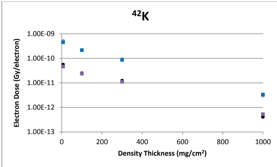
**Figure B-6** A Point Source Geometry Comparison of VARSKIN 5 (boxes) and VARSKIN 4 (circles) Predicted Dose Per Initial Beta From 42K as a Function of Density Thickness in Tissue and a Tissue Volume Cylinder of Area 1 cm<sup>2</sup> (upper) and 10 cm<sup>2</sup> (lower), With a Thickness of 20 mm
