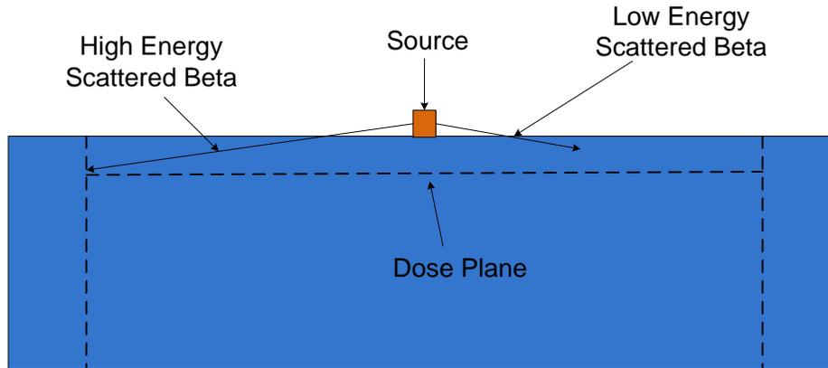
**Figure 3-8 Schematic Illustrating Electron Energy Limitations of Side-Scatter Corrections**
