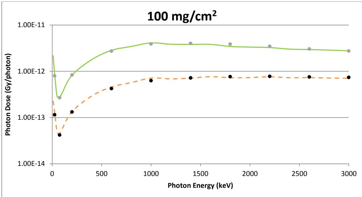
**Figure A-2** A Point Source Geometry Comparison of VARSKIN 5 (circles) and MCNP5 (lines) Predicted Dose Per Initial Photon as a Function of Photon Energy in Tissue at a Density Thickness of 100 mg/cm<sup>2</sup> and a Tissue Volume Cylinder of Area 1 cm<sup>2</sup> (solid line) and 10 cm<sup>2</sup> (dashed line), With a Thickness of 20 mm
