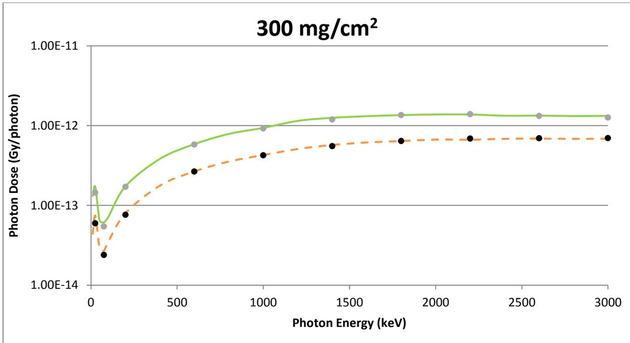
**Figure A-7** A Disk Source Geometry Comparison of VARSKIN 5 (circles) and MCNP5 (lines) Predicted Dose Per Initial Photon as a Function of Photon Energy in Tissue at a Density Thickness of 300 mg/cm<sup>2</sup> and a Tissue Volume Cylinder of Area 1 cm<sup>2</sup> (solid line) and 10 cm<sup>2</sup> (dashed line), With a Thickness of 20 mm
