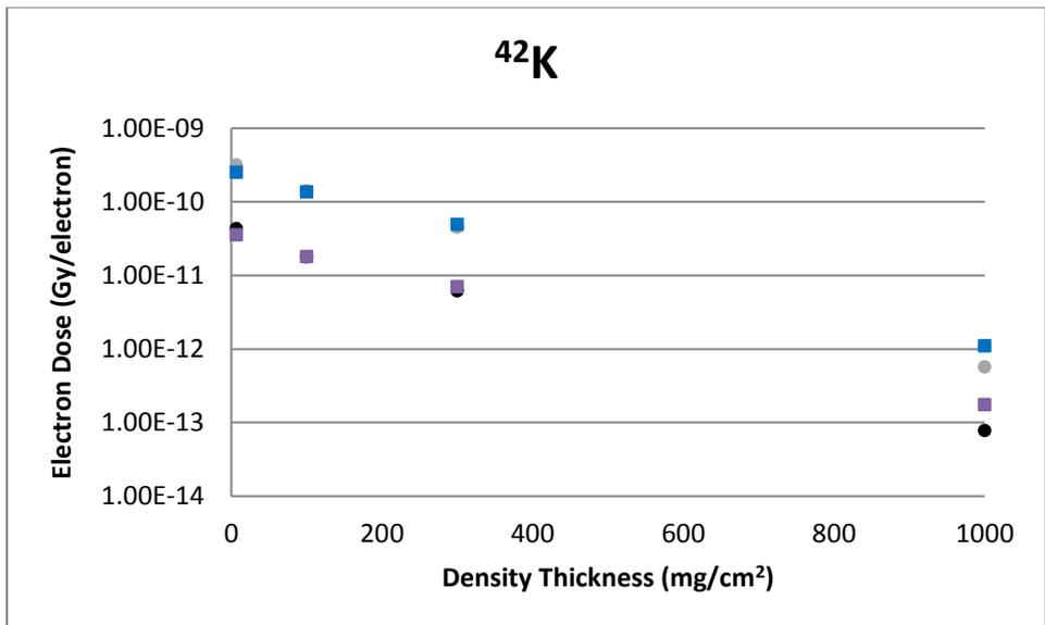
**Figure B-54** A Slab Source Geometry Comparison of VARSKIN 5 (boxes) and VARSKIN 4 (circles) Predicted Dose Per Initial Beta From <sup>42</sup>K as a Function of Density Thickness in Tissue and a Tissue Volume Cylinder of Area 1 cm<sup>2</sup> (upper) and 10 cm<sup>2</sup> (lower), With a Thickness of 20 mm
