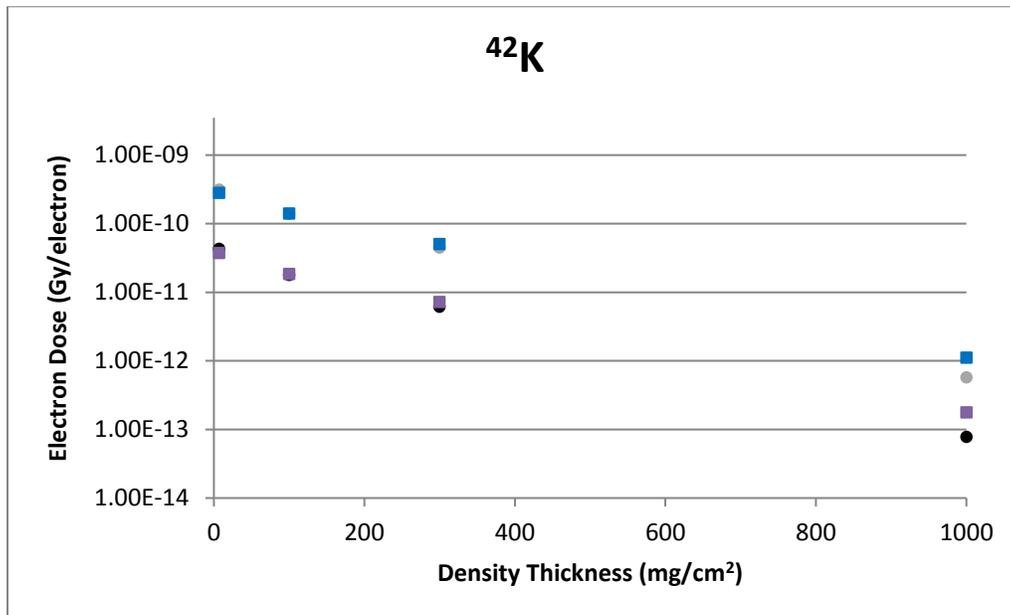
**Figure B-38** A Cylindrical Source Geometry Comparison of VARSKIN 5 (boxes) and VARSKIN 4 (circles) Predicted Dose Per Initial Beta From  $^{42}\text{K}$  as a Function of Density Thickness in Tissue and a Tissue Volume Cylinder of Area 1 cm<sup>2</sup> (upper) and 10 cm<sup>2</sup> (lower), With a Thickness of 20 mm
