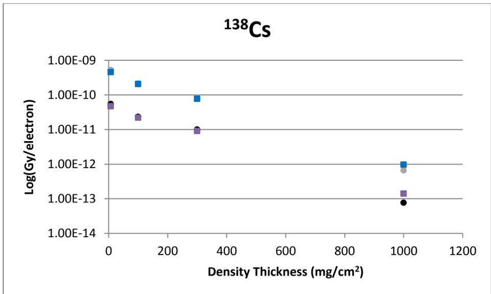
**Figure B-24** A 1 mm Diameter Disk Geometry Comparison of VARSKIN 5 (boxes) and VARSKIN 4 (circles) Predicted Dose Per Initial Beta From  $^{138}\text{Cs}$  as a Function of Density Thickness in Tissue and a Tissue Volume Cylinder of Area 1 cm<sup>2</sup> (upper) and 10 cm<sup>2</sup> (lower), With a Thickness of 20 mm
