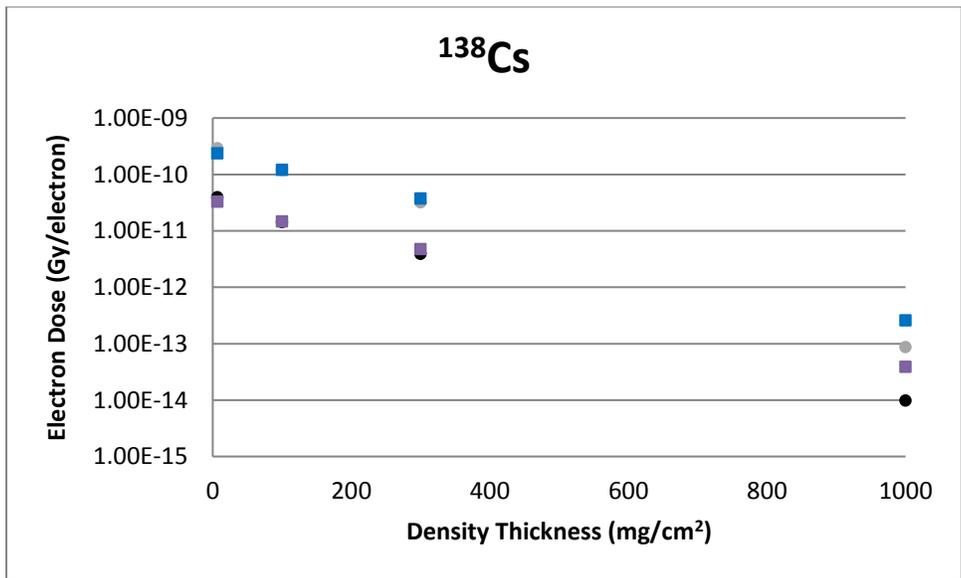
**Figure B-56** A Slab Source Geometry Comparison of VARSKIN 5 (boxes) and VARSKIN 4 (circles) Predicted Dose Per Initial Beta From  $^{138}\text{Cs}$  as a Function of Density Thickness in Tissue and a Tissue Volume Cylinder of Area 1 cm<sup>2</sup> (upper) and 10 cm<sup>2</sup> (lower), With a Thickness of 20 mm
