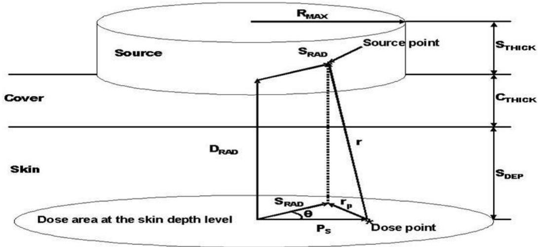
**Figure 3-27 Schematic of a Generic Dose Calculation for Cylindrical Geometry**
