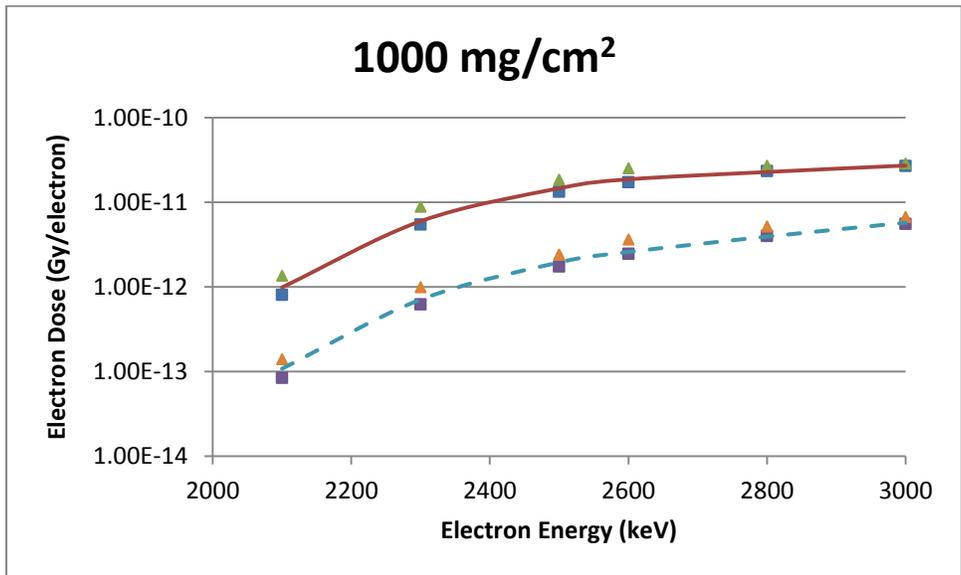
**Figure B-28** A 5 mm Diameter Disk Source Geometry Comparison of VARSKIN 5 (boxes), MCNP5 (triangles) and EGSnrc (lines) Predicted Dose Per Initial Electron as a Function of Electron Energy In Tissue at a Density Thickness of 1000 mg/cm<sup>2</sup> and a Tissue Volume Cylinder of Area 1 cm<sup>2</sup> (solid line) and 10 cm<sup>2</sup> (dashed line), With a Thickness of 20 mm
