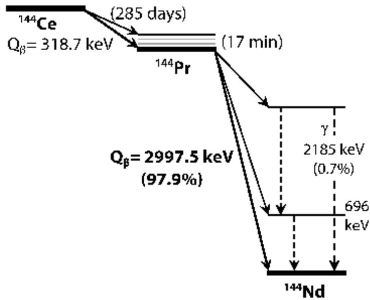
Figure C-1 The Decay Scheme of  $^{144}\text{Ce}$  to Stable  $^{144}\text{Nd}$
