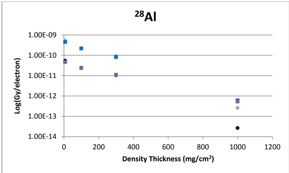
**Figure B-21** A 1 mm Diameter Disk Geometry Comparison of VARSKIN 5 (boxes) and VARSKIN 4 (circles) Predicted Dose Per Initial Beta From <sup>28</sup>Al as a Function of Density Thickness in Tissue and a Tissue Volume Cylinder of Area 1 cm<sup>2</sup> (upper) and 10 cm<sup>2</sup> (lower), With a Thickness of 20 mm
