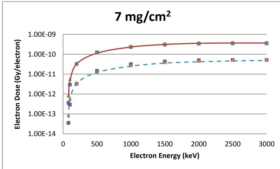
Figure B-49 A Slab Source Geometry Comparison of VARSKIN 5 (boxes), MCNP5 (triangles) and EGSnrc (lines) Predicted Dose Per Initial Electron as a Function of Electron Energy in Tissue at a Density Thickness of 7 mg/cm<sup>2</sup> and a Tissue Volume Cylinder of Area 1 cm<sup>2</sup> (solid line) and 10 cm<sup>2</sup> (dashed line), With a Thickness of 20 mm
