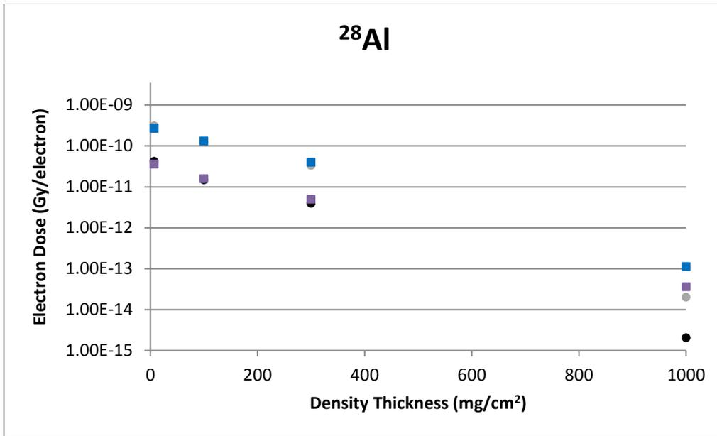
**Figure B-37** A Cylindrical Source Geometry Comparison of VARSKIN 5 (boxes) and VARSKIN 4 (circles) Predicted Dose Per Initial Beta From  $^{28}\text{Al}$  as a Function of Density Thickness in Tissue and a Tissue Volume Cylinder of Area 1 cm<sup>2</sup> (upper) and 10 cm<sup>2</sup> (lower), With a Thickness of 20 mm
