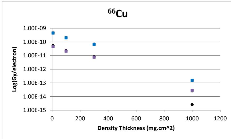
**Figure B-31** A 5 mm Diameter Disk Geometry Comparison of VARSKIN 5 (boxes) and VARSKIN 4 (circles) Predicted Dose Per Initial Beta From  $^{66}\text{Cu}$  as a Function of Density Thickness in Tissue and a Tissue Volume Cylinder of Area 1 cm<sup>2</sup> (upper) and 10 cm<sup>2</sup> (lower), With a Thickness of 20 mm
