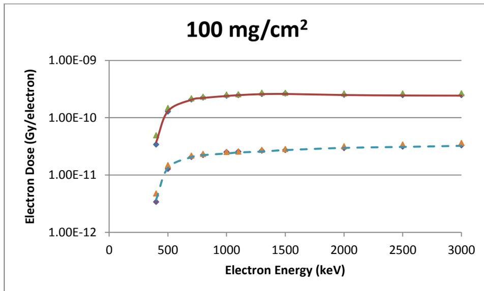
**Figure B-10** A 0.5 mm Diameter Disk Source Geometry Comparison of VARSKIN 5 (boxes), MCNP5 (triangles) and EGSnrc (lines) Predicted Dose Per Initial Electron as a Function of Electron Energy in Tissue at a Density Thickness of 100 mg/cm<sup>2</sup> and a Tissue Volume Cylinder of Area 1 cm<sup>2</sup> (solid line) and 10 cm<sup>2</sup> (dashed line), With a Thickness of 20 mm
