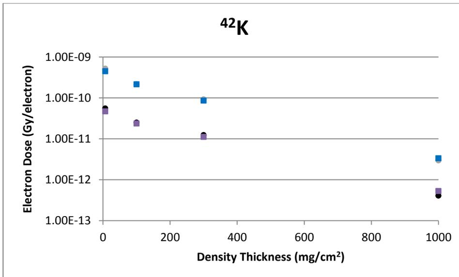
**Figure B-14** A 0.5 mm Diameter Disk Geometry Comparison of VARSKIN 5 (boxes) and VARSKIN 4 (circles) Predicted Dose Per Initial Beta From  $^{42}\text{K}$  as a Function of Density Thickness in Tissue and a Tissue Volume Cylinder of Area 1 cm<sup>2</sup> (upper) and 10 cm<sup>2</sup> (lower), With a Thickness of 20 mm
