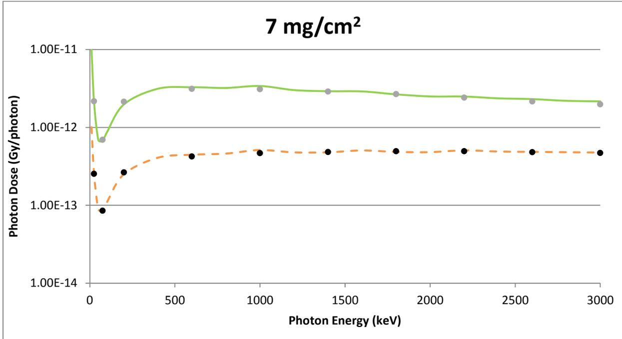
Figure A-1 A Point Source Geometry Comparison of VARSKIN 5 (Circles) and MCNP5 (lines) Predicted Dose Per Initial Photon as a Function of Photon Energy in Tissue at a Density Thickness of 7 mg/cm<sup>2</sup> and a Tissue Volume Cylinder of Area 1 cm<sup>2</sup> (solid line) and 10 cm<sup>2</sup>
