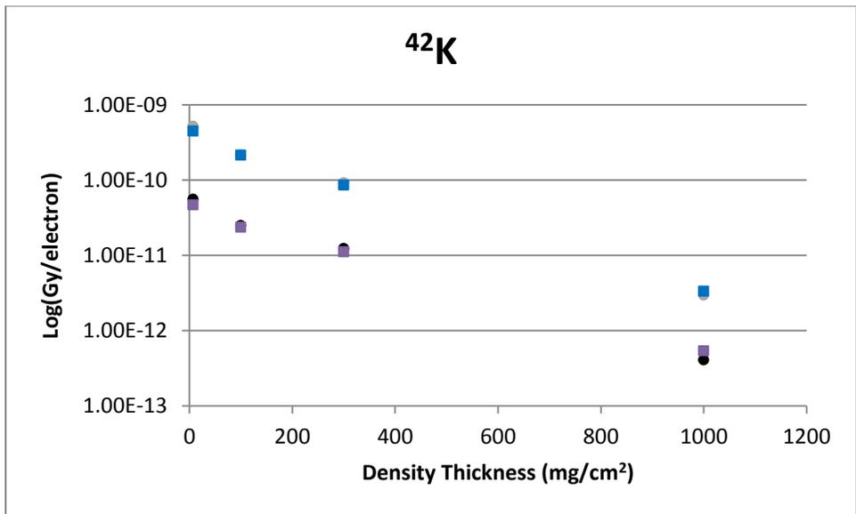
**Figure B-22** A 1 mm Diameter Disk Geometry Comparison of VARSKIN 5 (boxes) and VARSKIN 4 (circles) Predicted Dose Per Initial Beta From <sup>42</sup>K as a Function of Density Thickness in Tissue and a Tissue Volume Cylinder of Area 1 cm<sup>2</sup> (upper) and 10 cm<sup>2</sup> (lower), With a Thickness of 20 mm
