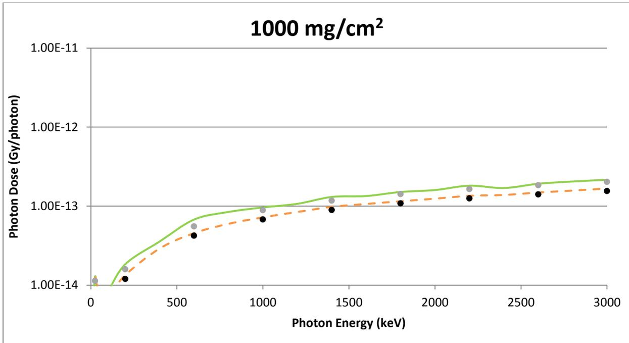
**Figure A-24 A Point Source Geometry With a Cotton Cover and a 1 cm Air Gap Comparison of VARSKIN 5 (circles) and MCNP5 (lines) Predicted Dose Per Initial Photon as a Function of Photon Energy in Tissue at a Density Thickness of 1000 mg/cm<sup>2</sup> and a Tissue Volume Cylinder of Area 1 cm<sup>2</sup> (solid line) and 10 cm<sup>2</sup> (dashed line); Thickness of 20 mm**
