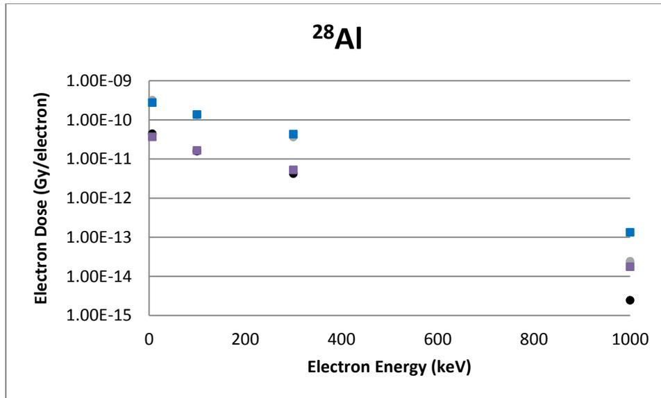
**Figure B-45** A Spherical Source Geometry Comparison of VARSKIN 5 (boxes) and VARSKIN 4 (circles) Predicted Dose Per Initial Beta From <sup>28</sup>Al as a Function of Density Thickness in Tissue and a Tissue Volume Cylinder of Area 1 cm<sup>2</sup> (upper) and 10 cm<sup>2</sup> (lower), With a Thickness of 20 mm
