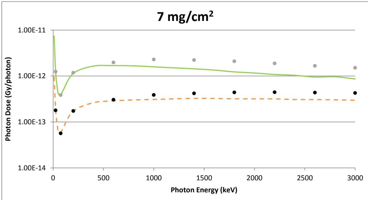
**Figure A-17** A Spherical Source Geometry Comparison of VARSKIN 5 (circles) and MCNP5 (Lines) Predicted Dose Per Initial Photon as a Function of Photon Energy in Tissue at a Density Thickness of 7 mg/cm<sup>2</sup> and a Tissue Volume Cylinder of Area 1 cm<sup>2</sup> (solid line) and 10 cm<sup>2</sup> (dashed line), With a Thickness of 20 mm
