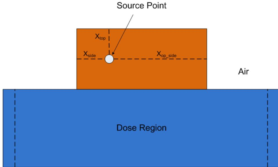
**Figure 3-11 Schematic Demonstrating Conditions for Air-Water Scattering Correction**
