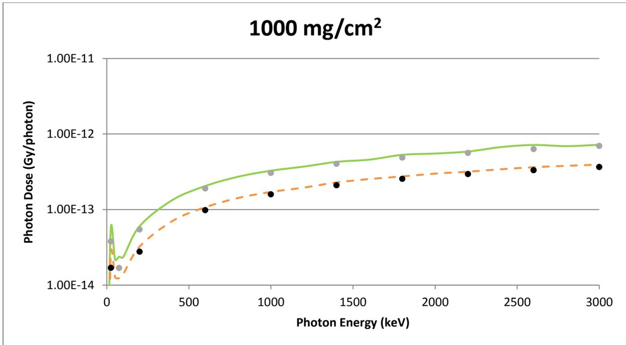
**Figure A-20** A Spherical Source Geometry Comparison of VARSKIN 5 (circles) and MCNP5 (lines) Predicted Dose Per Initial Photon as a Function of Photon Energy in Tissue at a Density Thickness of 1000 mg/cm<sup>2</sup> and a Tissue Volume Cylinder of Area 1 cm<sup>2</sup> (solid line) and 10 cm<sup>2</sup> (dashed line), With a Thickness of 20 mm
