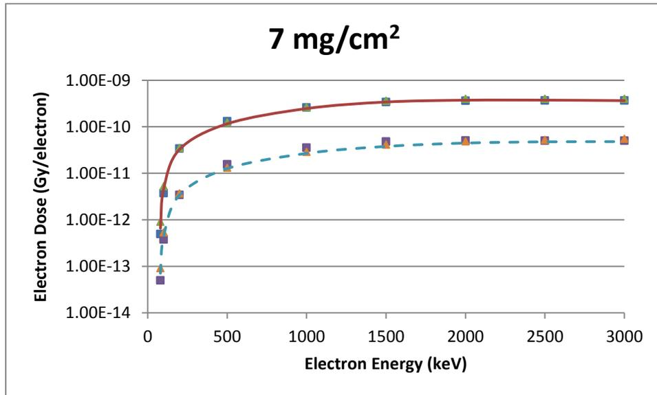
Figure B-41 A Spherical Source Geometry Comparison of VARSKIN 5 (boxes), MCNP5 (triangles) and EGSnrc (lines) Predicted Dose Per Initial Electron as a Function of Electron Energy in Tissue at a Density Thickness of 7 mg/cm<sup>2</sup> and a Tissue Volume Cylinder of Area 1 cm<sup>2</sup> (solid line) and 10 cm<sup>2</sup> (dashed line), With a Thickness of 20 mm
