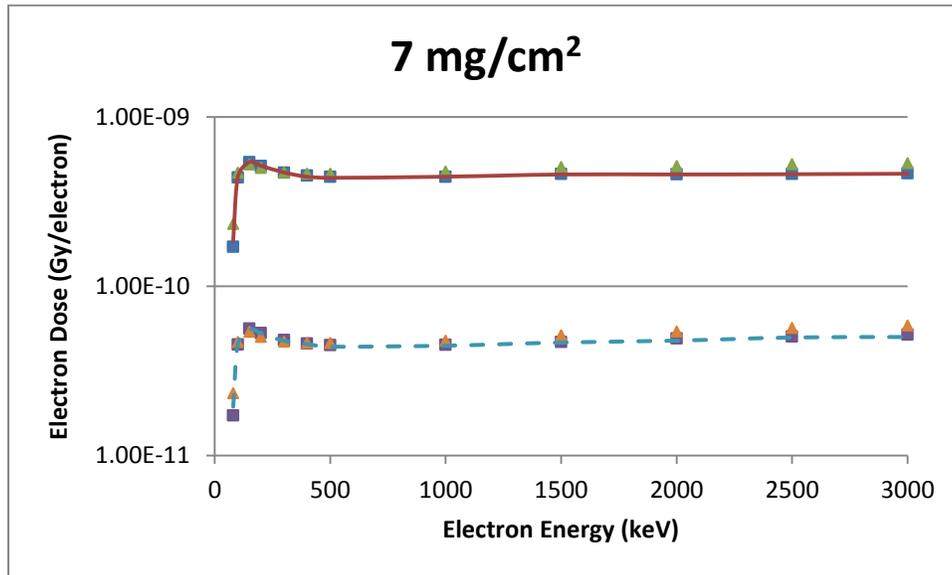
**Figure B-9** A 0.5 mm Diameter Disk Source Geometry Comparison of VARSKIN 5 (boxes), MCNP5 (triangles) And EGSnrc (lines) Predicted Dose Per Initial Electron as a Function of Electron Energy in Tissue at a Density Thickness of 7 mg/cm<sup>2</sup> and a Tissue Volume Cylinder of Area 1 cm<sup>2</sup> (solid line) and 10 cm<sup>2</sup> (dashed line), With a Thickness of 20 mm
