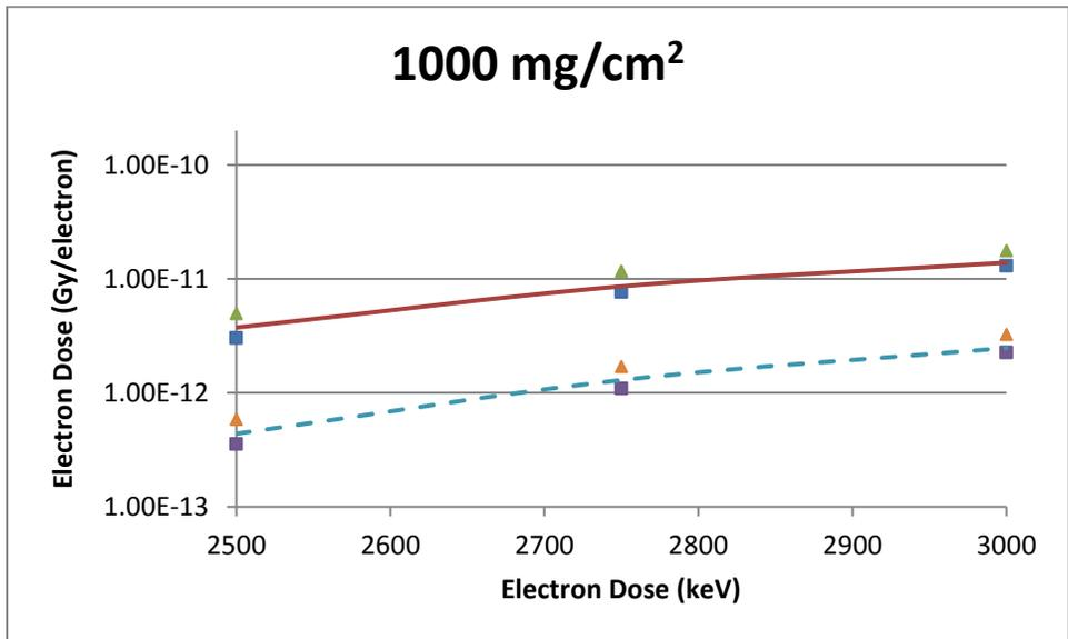
**Figure B-36** A Cylindrical Source Geometry Comparison of VARSKIN 5 (boxes), MCNP5 (triangles) and EGSnrc (lines) Predicted Dose Per Initial Electron as a Function of Electron Energy in Tissue at a Density Thickness of 1000 mg/cm<sup>2</sup> and a Tissue Volume Cylinder of Area 1 cm<sup>2</sup> (solid line) and 10 cm<sup>2</sup> (dashed line), With a Thickness of 20 mm
