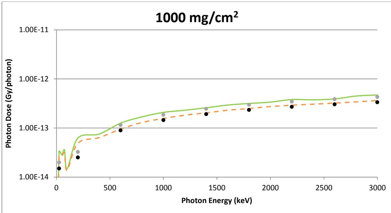
**Figure A-27** A Point Source Geometry 1 cm Off-Axis Comparison of VARSKIN 5 (circles) and MCNP5 (lines) Predicted Dose Per Initial Photon as a Function of Photon Energy in Tissue at a Density Thickness of 1000 mg/cm<sup>2</sup> and a Tissue Volume Cylinder of Area 1 cm<sup>2</sup> (solid line) and 10 cm<sup>2</sup> (dashed line), With a Thickness of 20 mm
