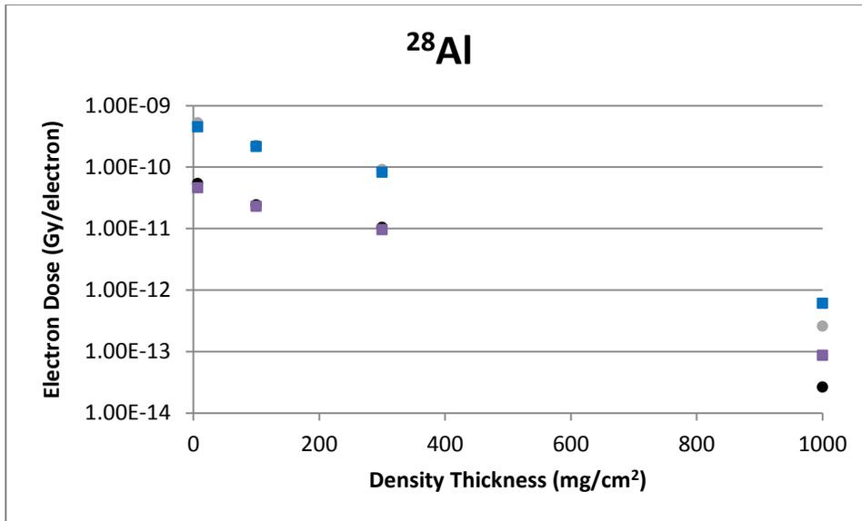
**Figure B-13** A 0.5 mm Diameter Disk Geometry Comparison of VARSKIN 5 (boxes) and VARSKIN 4 (circles) Predicted Dose Per Initial Beta From  $^{28}\text{Al}$  as a Function of Density Thickness in Tissue and a Tissue Volume Cylinder of Area 1 cm<sup>2</sup> (upper) and 10 cm<sup>2</sup> (lower), With a Thickness of 20 mm
