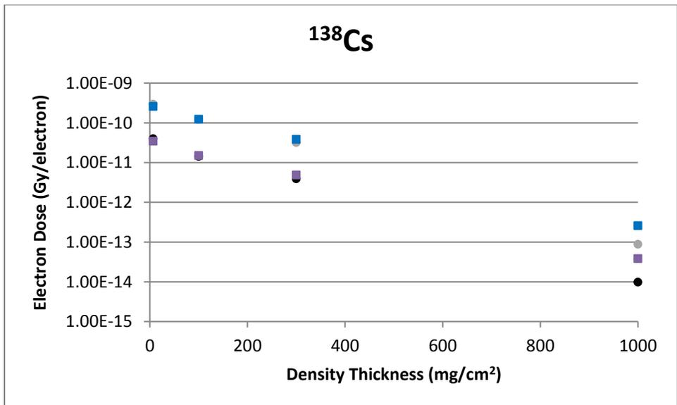
**Figure B-40** A Cylindrical Source Geometry Comparison of VARSKIN 5 (boxes) and VARSKIN 4 (circles) Predicted Dose Per Initial Beta From <sup>138</sup>Cs as a Function of Density Thickness in Tissue and a Tissue Volume Cylinder of Area 1 cm<sup>2</sup> (upper) and 10 cm<sup>2</sup> (lower), With a Thickness of 20 mm
