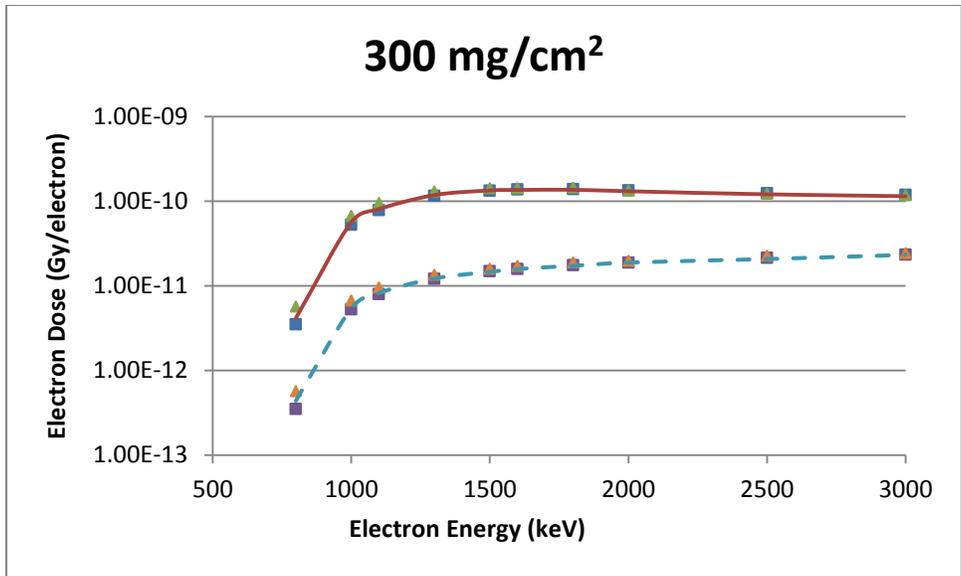
**Figure B-27** A 5 mm Diameter Disk Source Geometry Comparison of VARSKIN 5 (boxes), MCNP5 (triangles) and EGSnrc (lines) Predicted Dose Per Initial Electron as a Function of Electron Energy in Tissue at a Density Thickness of 300 mg/cm<sup>2</sup> and a Tissue Volume Cylinder of Area 1 cm<sup>2</sup> (solid line) and 10 cm<sup>2</sup> (dashed line), With a Thickness of 20 mm
