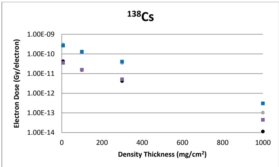
**Figure B-48** A Spherical Source Geometry Comparison of VARSKIN 5 (boxes) and VARSKIN 4 (circles) Predicted Dose Per Initial Beta From  $^{138}\text{Cs}$  as a Function of Density Thickness in Tissue and a Tissue Volume Cylinder of Area 1 cm<sup>2</sup> (upper) and 10 cm<sup>2</sup> (lower), With a Thickness of 20 mm
