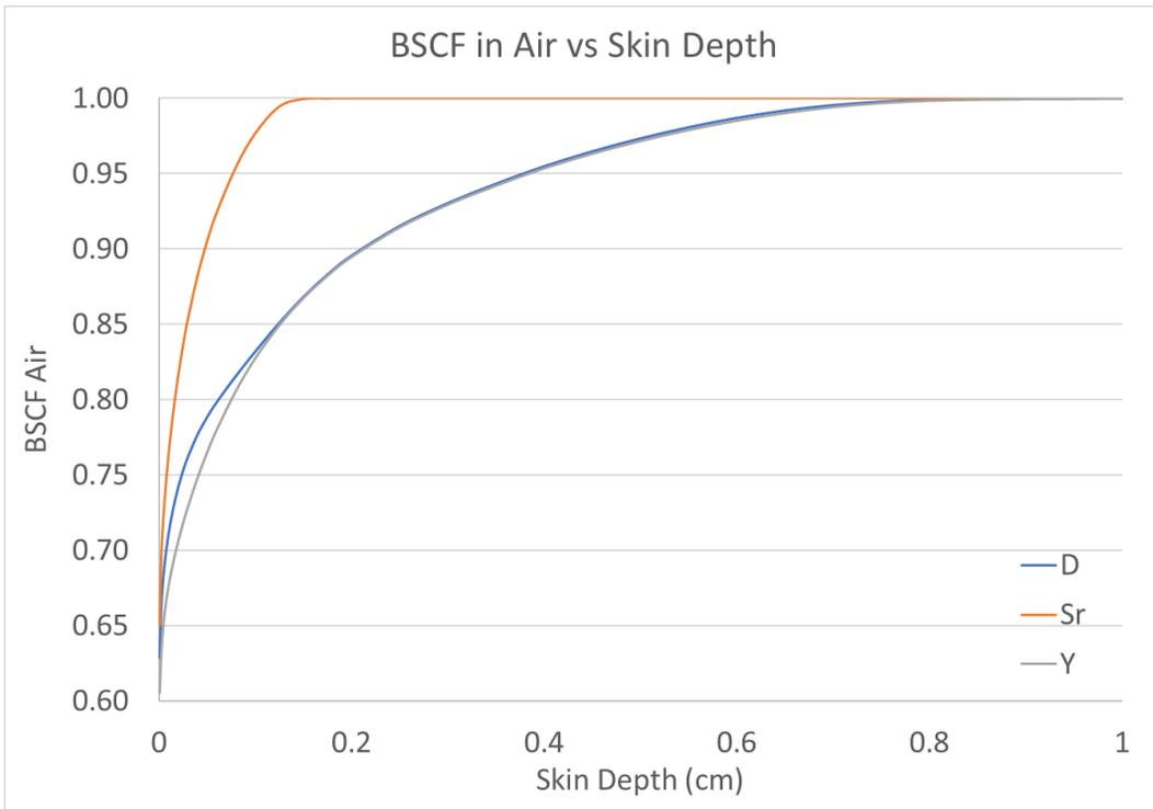
**Figure 5-1 Backscatter Factors in Air as a Function of Depth in Tissue**
