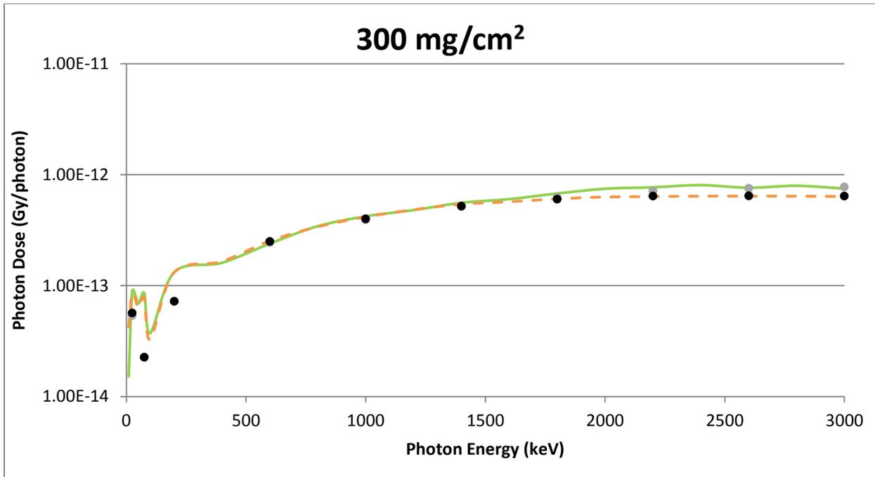
**Figure A-26** A Point Source Geometry 1 cm Off-Axis Comparison of VARSKIN 5 (circles) and MCNP5 (lines) Predicted Dose Per Initial Photon as a Function of Photon Energy in Tissue at a Density Thickness of 300 mg/cm<sup>2</sup> and a Tissue Volume Cylinder of Area 1 cm<sup>2</sup> (solid line) and 10 cm<sup>2</sup> (dashed line), With a Thickness of 20 mm
