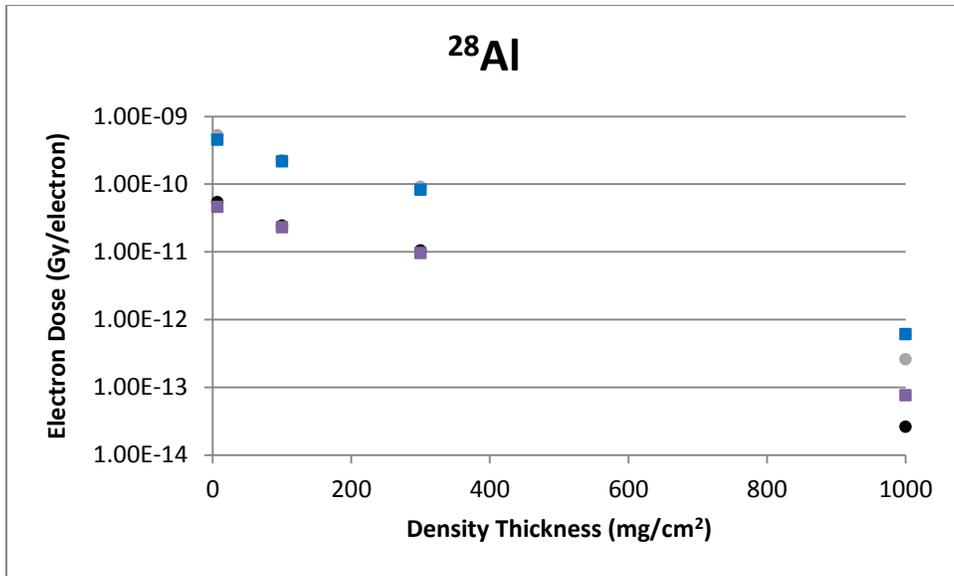
**Figure B-5** A Point Source Geometry Comparison of VARSKIN 5 (boxes) and VARSKIN 4 (circles) Predicted Dose Per Initial Beta From  $^{28}\text{Al}$  as a Function of Density Thickness in Tissue and a Tissue Volume Cylinder of Area 1 cm<sup>2</sup> (upper) and 10 cm<sup>2</sup> (lower), With a Thickness of 20 mm
