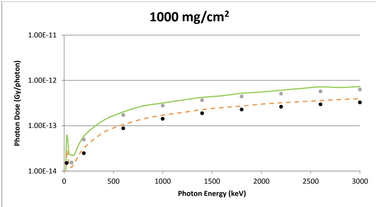
**Figure A-16** A Slab Source Geometry Comparison of VARSKIN 5 (circles) and MCNP5 (lines) Predicted Dose Per Initial Photon as a Function of Photon Energy in Tissue at a Density Thickness of 1000 mg/cm<sup>2</sup> and a Tissue Volume Cylinder of Area 1 cm<sup>2</sup> (solid line) and 10 cm<sup>2</sup> (dashed line), With a Thickness of 20 mm
