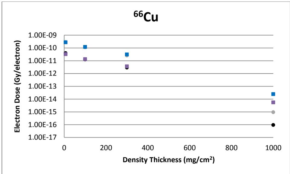
**Figure B-47** A Spherical Source Geometry Comparison of VARSKIN 5 (boxes) and VARSKIN 4 (circles) Predicted Dose Per Initial Beta From  $^{66}\text{Cu}$  as a Function of Density Thickness in Tissue and a Tissue Volume Cylinder of Area 1 cm<sup>2</sup> (upper) and 10 cm<sup>2</sup> (lower), With a Thickness of 20 mm
