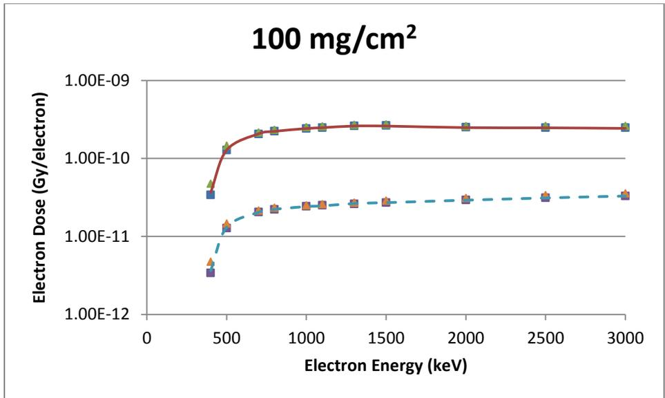
**Figure B-2** A Point Source Geometry Comparison of VARSKIN 5 (boxes), MCNP5 (triangles) and EGSnrc (lines) Predicted Dose Per Initial Electron as a Function of Electron Energy in Tissue at a Density Thickness of 100 mg/cm<sup>2</sup> and a 20 mm Thick Tissue Volume Cylinder of Area 1 cm<sup>2</sup> (solid line) and 10 cm<sup>2</sup> (dashed line)
