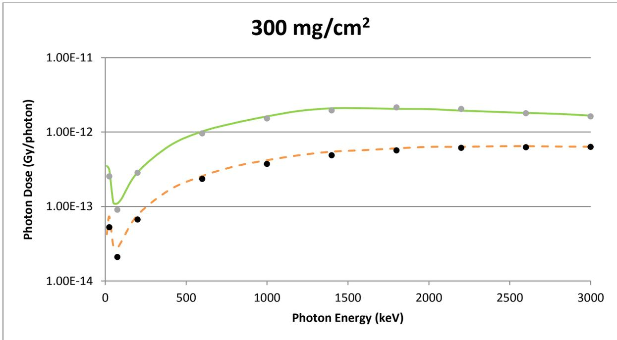
**Figure A-15** A Slab Source Geometry Comparison of VARSKIN 5 (circles) and MCNP5 (lines) Predicted Dose Per Initial Photon as a Function of Photon Energy in Tissue at a Density Thickness of 300 mg/cm<sup>2</sup> and a Tissue Volume Cylinder of Area 1 cm<sup>2</sup> (solid line) and 10 cm<sup>2</sup> (dashed line), With a Thickness of 20 mm
