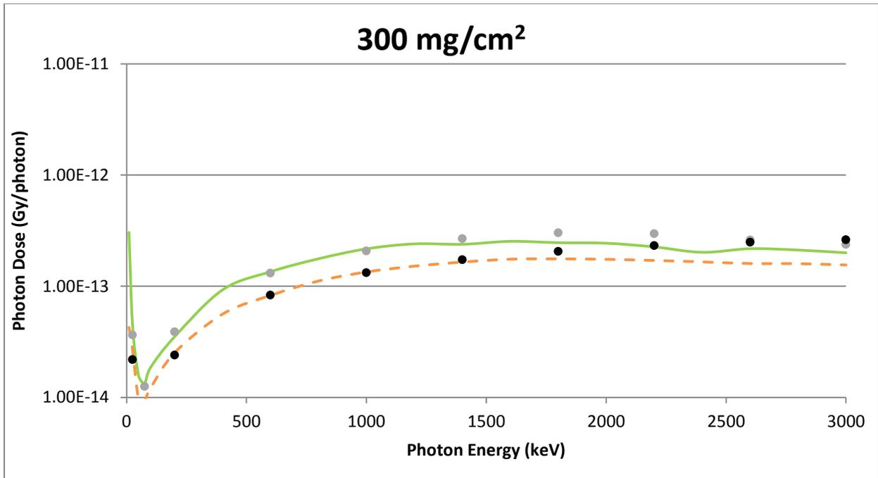
**Figure A-23 A Point Source Geometry With a Cotton Cover and a 1 cm Air Gap Comparison of VARSKIN 5 (circles) and MCNP5 (lines) Predicted Dose Per Initial Photon as a Function of Photon Energy in Tissue at a Density Thickness of 300 mg/cm<sup>2</sup> and a Tissue Volume Cylinder of Area 1 cm<sup>2</sup> (solid line) and 10 cm<sup>2</sup> (dashed line); Thickness of 20 mm**
