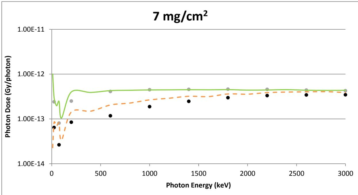
**Figure A-25 A Point Source Geometry 1 cm Off-Axis Comparison of VARSKIN 5 (circles) and MCNP5 (lines) Predicted Dose Per Initial Photon as a Function of Photon Energy in Tissue at a Density Thickness of  $7 \text{ mg/cm}^2$  and a Tissue Volume Cylinder of Area  $1 \text{ cm}^2$  (solid line) and  $10 \text{ cm}^2$  (dashed line), With a Thickness of 20 mm**
