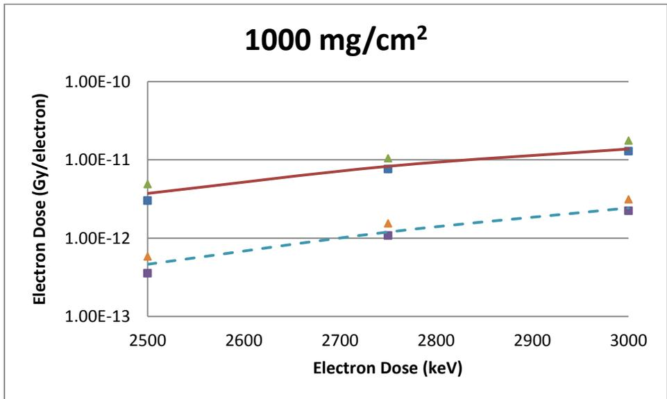
**Figure B-52** A Slab Source Geometry Comparison of VARSKIN 5 (boxes), MCNP5 (triangles) and EGSnrc (lines) Predicted Dose Per Initial Electron as a Function of Electron Energy in Tissue at a Density Thickness of 1000 mg/cm<sup>2</sup> and a Tissue Volume Cylinder of Area 1 cm<sup>2</sup> (solid line) and 10 cm<sup>2</sup> (dashed line), With a Thickness of 20 mm
