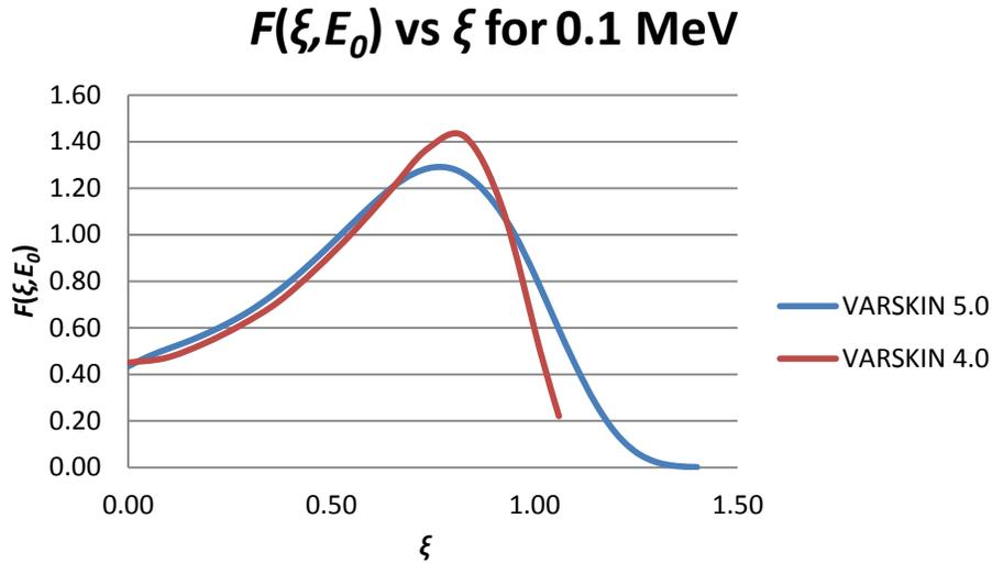
**Figure 3-1 Scaled Absorbed Dose Distributions for 0.1 Mev Electrons**
