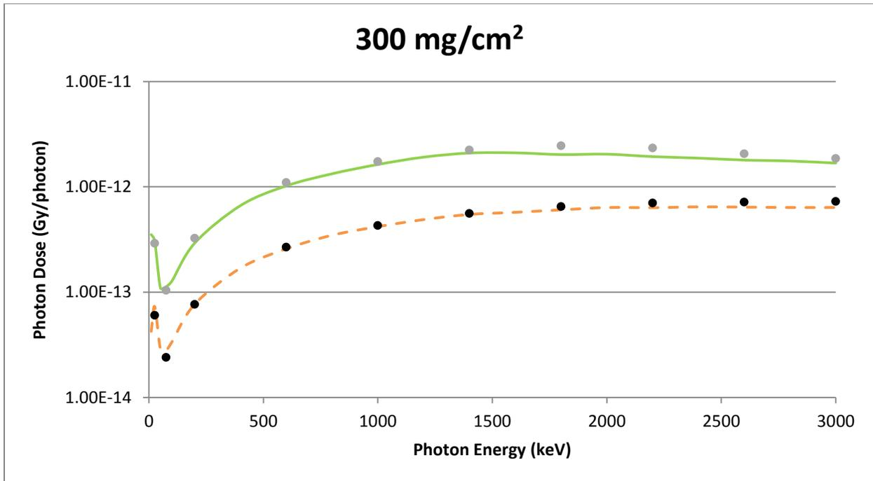
**Figure A-11** A Cylindrical Source Geometry Comparison of VARSKIN 5 (circles) and MCNP5 (lines) Predicted Dose Per Initial Photon as a Function of Photon Energy in Tissue at a Density Thickness of 300 mg/cm<sup>2</sup> and a Tissue Volume Cylinder of Area 1 cm<sup>2</sup> (solid line) and 10 cm<sup>2</sup> (dashed line), With a Thickness of 20 mm
