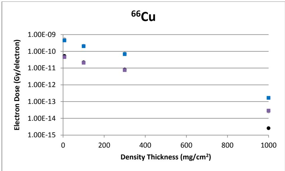
**Figure B-15** A 0.5 mm Diameter Disk Geometry Comparison of VARSKIN 5 (boxes) and VARSKIN 4 (circles) Predicted Dose Per Initial Beta From  $^{66}\text{Cu}$  as a Function of Density Thickness in Tissue and a Tissue Volume Cylinder of Area 1 cm<sup>2</sup> (upper) and 10 cm<sup>2</sup> (lower), With a Thickness of 20 mm
