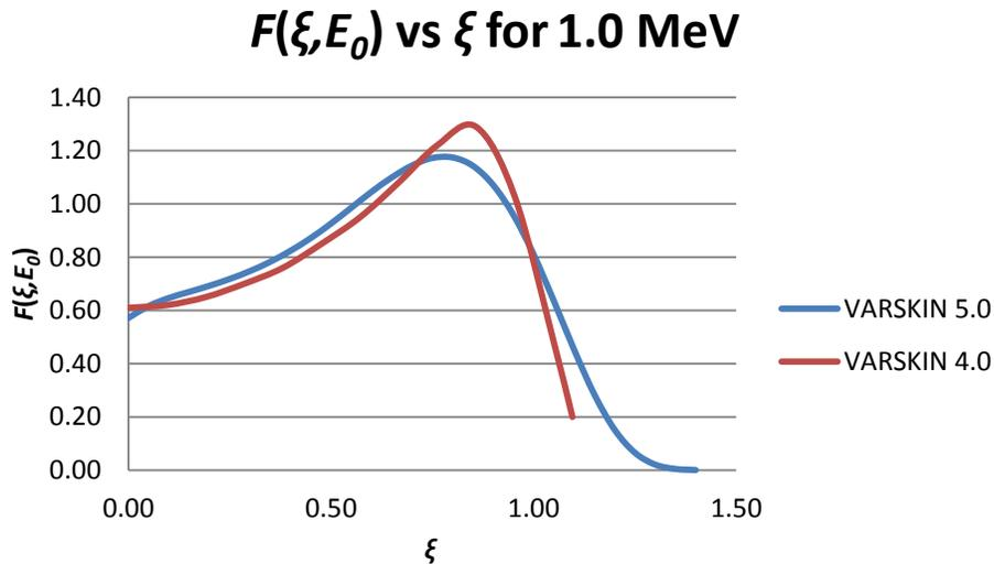
**Figure 3-2 Scaled Absorbed Dose Distributions for 1.0 Mev Electrons**
