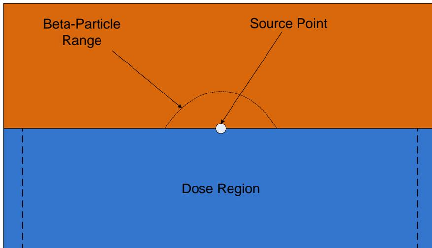
**Figure 3-6 Schematic Demonstrating Conditions for Full Source-Water Scattering**
