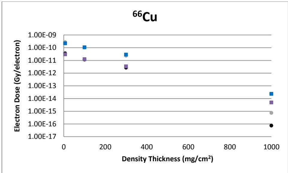
**Figure B-55** A Slab Source Geometry Comparison of VARSKIN 5 (boxes) and VARSKIN 4 (circles) Predicted Dose Per Initial Beta From  $^{66}\text{Cu}$  as a Function of Density Thickness in Tissue and a Tissue Volume Cylinder of Area 1 cm<sup>2</sup> (upper) and 10 cm<sup>2</sup> (lower), With a Thickness of 20 mm
