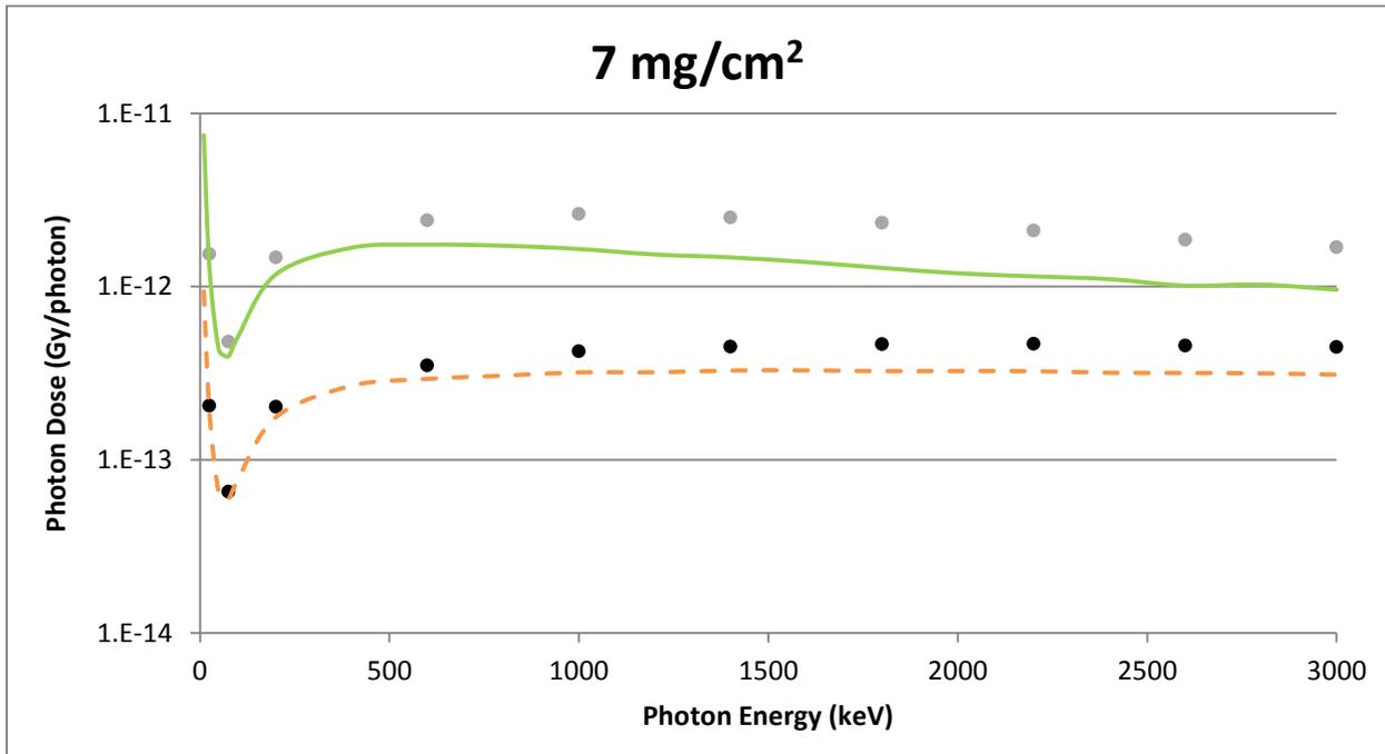
**Figure A-9** A Cylindrical Source Geometry Comparison of VARSKIN 5 (circles) and MCNP5 (lines) Predicted Dose Per Initial Photon as a Function of Photon Energy in Tissue at a Density Thickness of 7 mg/cm<sup>2</sup> and a Tissue Volume Cylinder of Area 1 cm<sup>2</sup> (solid line) and 10 cm<sup>2</sup> (dashed line), With a Thickness of 20 mm
