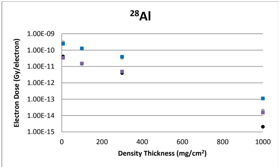
**Figure B-53** A Slab Source Geometry Comparison of VARSKIN 5 (boxes) and VARSKIN 4 (circles) Predicted Dose Per Initial Beta From <sup>28</sup>Al as a Function of Density Thickness in Tissue and a Tissue Volume Cylinder of Area 1 cm<sup>2</sup> (upper) and 10 cm<sup>2</sup> (lower), With a Thickness of 20 mm
