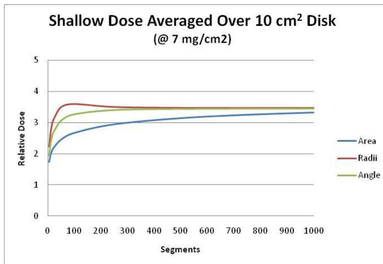
**Figure 3-21 Relative Dose as a Function of the Number of Segments in a Numerical Integration**
