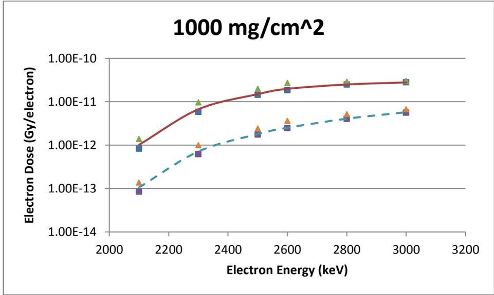
**Figure B-12** A 0.5 mm Diameter Disk Source Geometry Comparison of VARSKIN 5 (boxes), MCNP5 (triangles) and EGSnrc (lines) Predicted Dose Per Initial Electron as a Function of Electron Energy in Tissue at a Density Thickness of 1000 mg/cm<sup>2</sup> and a Tissue Volume Cylinder of Area 1 cm<sup>2</sup> (solid line) and 10 cm<sup>2</sup> (dashed line), With a Thickness of 20 mm
