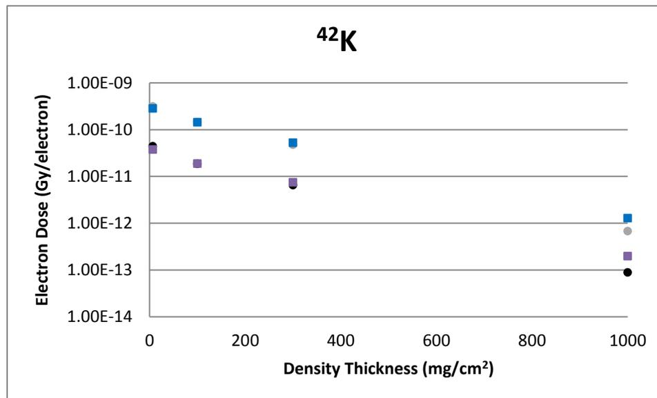
**Figure B-46** A Spherical Source Geometry Comparison of VARSKIN 5 (boxes) and VARSKIN 4 (circles) Predicted Dose Per Initial Beta From <sup>42</sup>K as a Function of Density Thickness in Tissue and a Tissue Volume Cylinder of Area 1 cm<sup>2</sup> (upper) and 10 cm<sup>2</sup> (lower), With a Thickness of 20 mm
