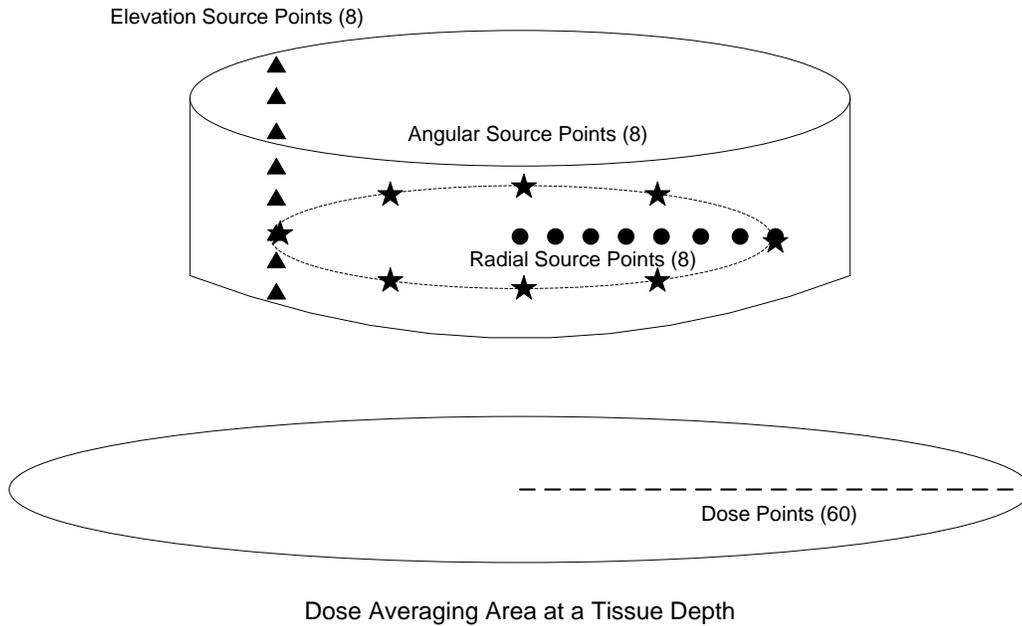
**Figure 3-3 Schematic of the Eight-Panel Quadrature Routine (redrawn from Durham 2006)**
