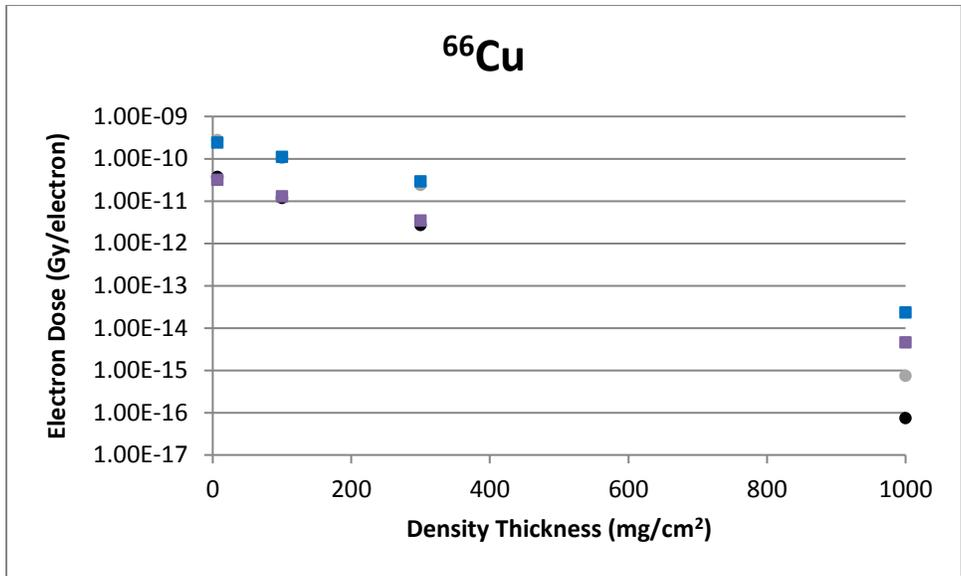
**Figure B-39** A Cylindrical Source Geometry Comparison of VARSKIN 5 (boxes) and VARSKIN 4 (circles) Predicted Dose Per Initial Beta From <sup>66</sup>Cu as a Function of Density Thickness in Tissue and a Tissue Volume Cylinder of Area 1 cm<sup>2</sup> (upper) and 10 cm<sup>2</sup> (lower), With a Thickness of 20 mm
