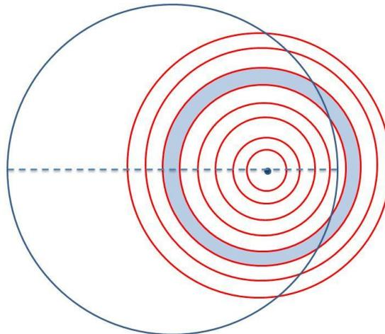
**Figure 3-24 Dose-Averaging Disk with the Source Point Located off Axis, on Disk**
