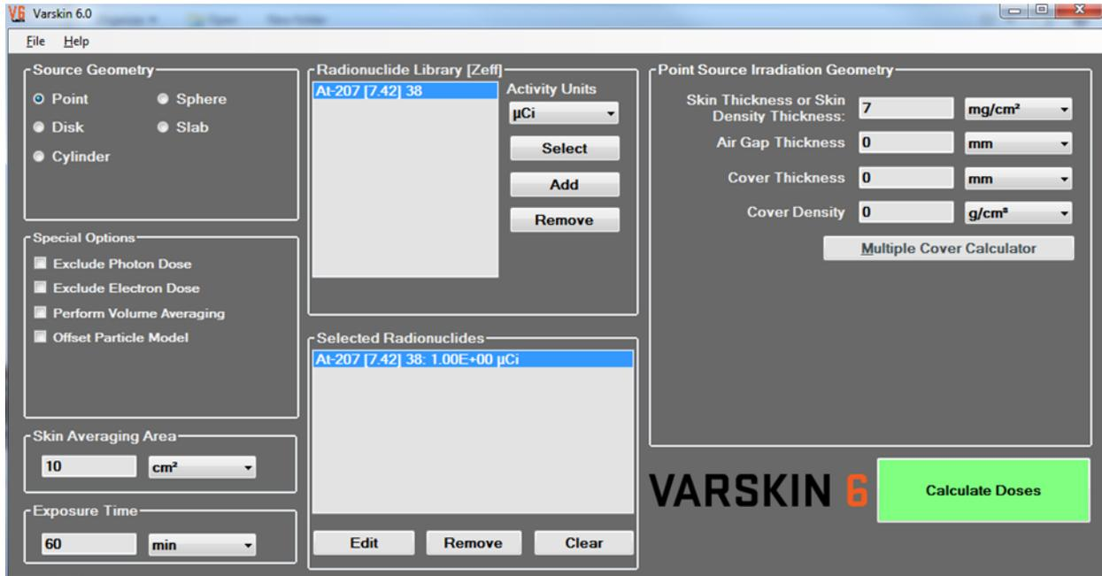
Figure 2-1 Initial View and Main Input Window (Source Geometry option box in upper left corner)
