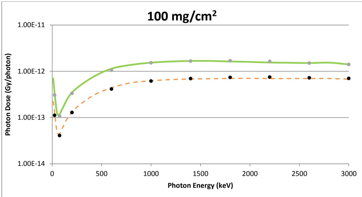
**Figure A-6** A Disk Source Geometry Comparison of VARSKIN 5 (circles) and MCNP5 (Lines) Predicted Dose Per Initial Photon as a Function of Photon Energy in Tissue at a Density Thickness of 100 mg/cm<sup>2</sup> and a Tissue Volume Cylinder of Area 1 cm<sup>2</sup> (solid line) and 10 cm<sup>2</sup> (dashed line), With a Thickness of 20 mm
