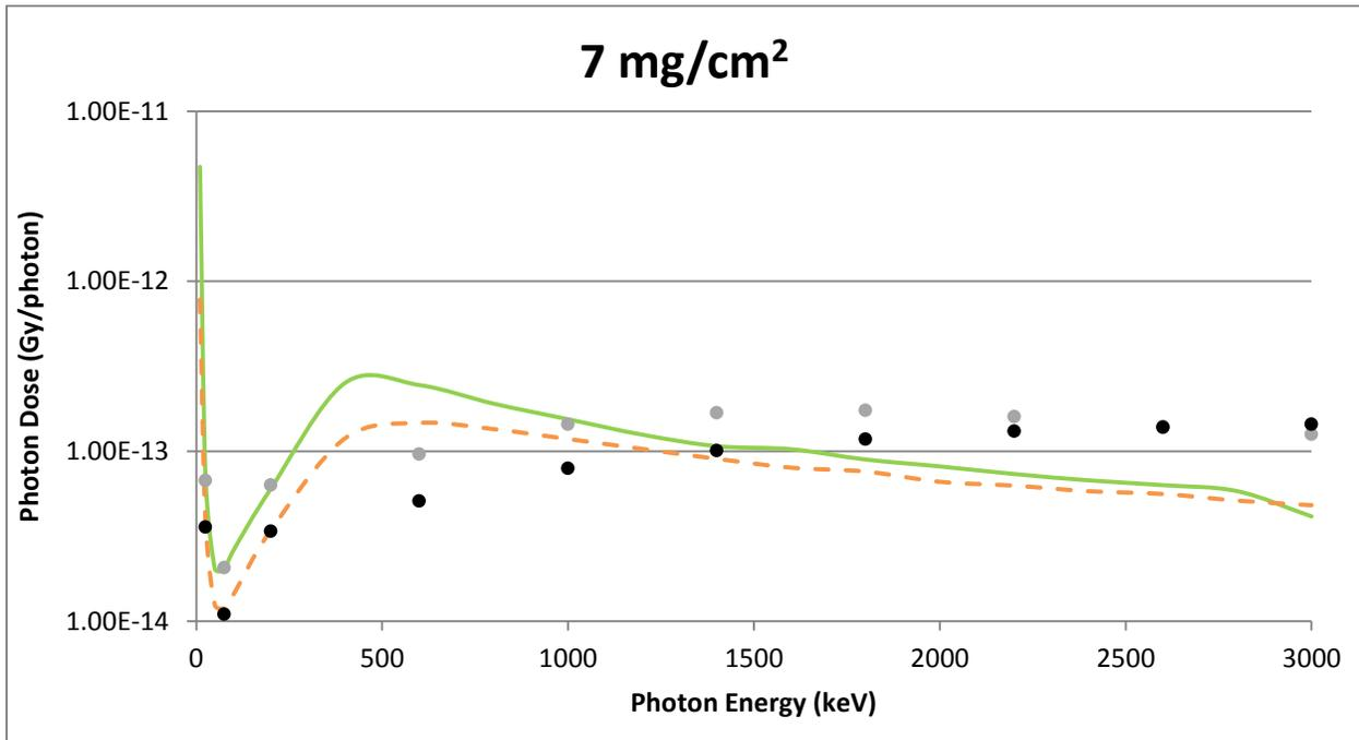
**Figure A-21 A Point Source Geometry With a Cotton Cover and a 1 cm Air Gap Comparison of VARSKIN 5 (circles) and MCNP5 (lines) Predicted Dose Per Initial Photon as a Function of Photon Energy in Tissue at a Density Thickness of 7 mg/cm<sup>2</sup> and a Tissue Volume Cylinder of Area 1 cm<sup>2</sup> (solid line) and 10 cm<sup>2</sup> (dashed line); Thickness of 20 mm**
