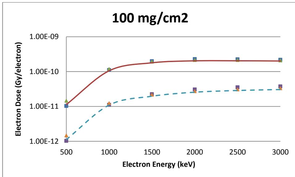
Figure B-42 A Spherical Source Geometry Comparison of VARSKIN 5 (boxes), MCNP5 (triangles) and EGSnrc (lines) Predicted Dose Per Initial Electron as a Function of Electron Energy in Tissue at a Density Thickness of 100 mg/cm<sup>2</sup> and a Tissue Volume Cylinder of Area 1 cm<sup>2</sup> (solid line) and 10 cm<sup>2</sup> (dashed line), With a Thickness of 20 mm
