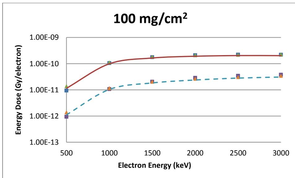
Figure B-50 A Slab Source Geometry Comparison of VARSKIN 5 (boxes), MCNP5 (triangles) and EGSnrc (lines) Predicted Dose Per Initial Electron as a Function of Electron Energy in Tissue at a Density Thickness of 100 mg/cm<sup>2</sup> and a Tissue Volume Cylinder of Area 1 cm<sup>2</sup> (solid line) and 10 cm<sup>2</sup> (dashed line), With a Thickness of 20 mm
