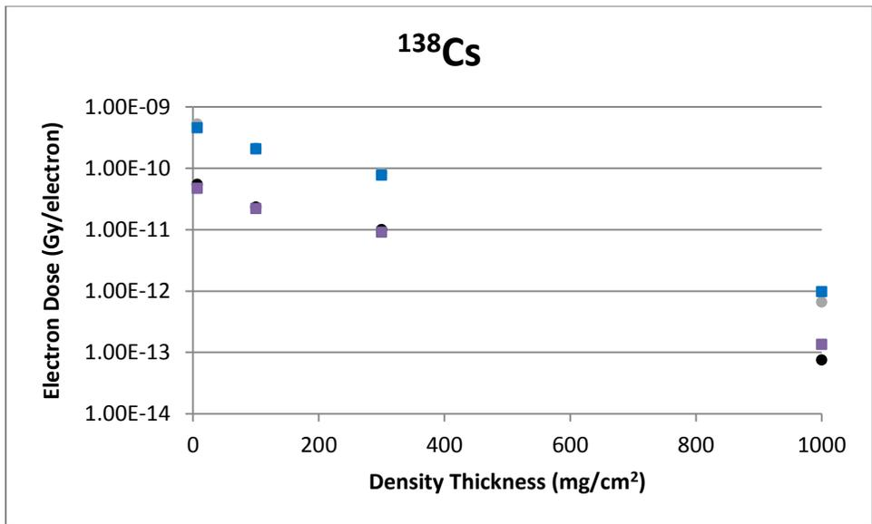
**Figure B-16** A 0.5 mm Diameter Disk Geometry Comparison of VARSKIN 5 (boxes) and VARSKIN 4 (circles) Predicted Dose Per Initial Beta From  $^{138}\text{Cs}$  as a Function of Density Thickness in Tissue and a Tissue Volume Cylinder of Area 1 cm<sup>2</sup> (upper) and 10 cm<sup>2</sup> (lower), With a Thickness of 20 mm
