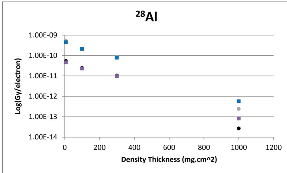
**Figure B-29** A 5 mm Diameter Disk Geometry Comparison of VARSKIN 5 (boxes) and VARSKIN 4 (circles) Predicted Dose Per Initial Beta From  $^{28}\text{Al}$  as a Function of Density Thickness in Tissue and a Tissue Volume Cylinder of Area 1 cm<sup>2</sup> (upper) and 10 cm<sup>2</sup> (lower), With a Thickness of 20 mm
