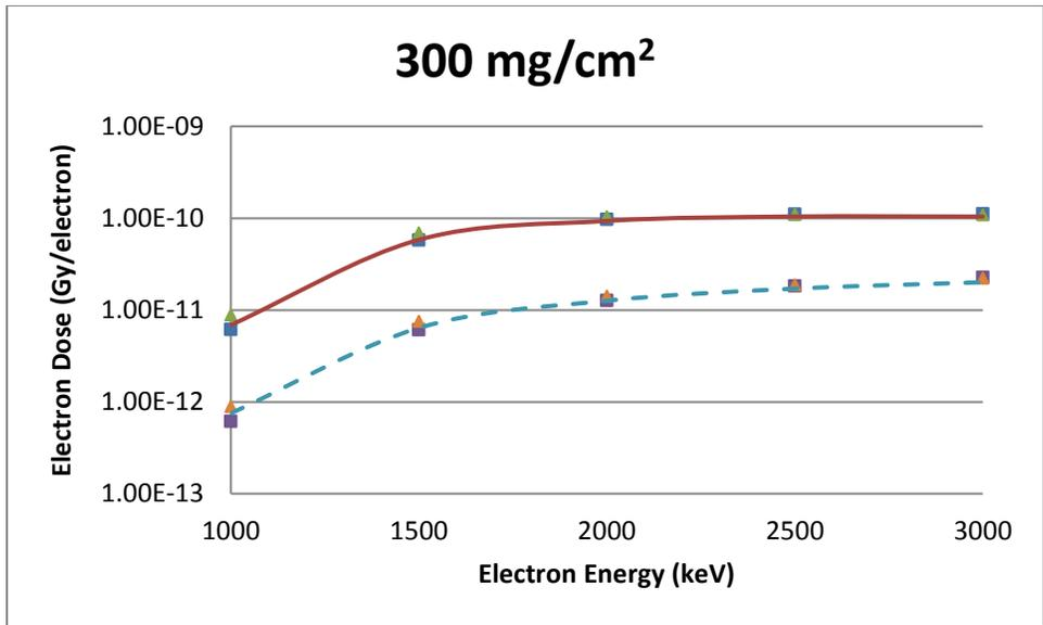
**Figure B-51** A Slab Source Geometry Comparison of VARSKIN 5 (boxes), MCNP5 (triangles) and EGSnrc (lines) Predicted Dose Per Initial Electron as a Function of Electron Energy in Tissue at a Density Thickness of 300 mg/cm<sup>2</sup> and a Tissue Volume Cylinder of Area 1 cm<sup>2</sup> (solid line) and 10 cm<sup>2</sup> (dashed line), With a Thickness of 20 mm
