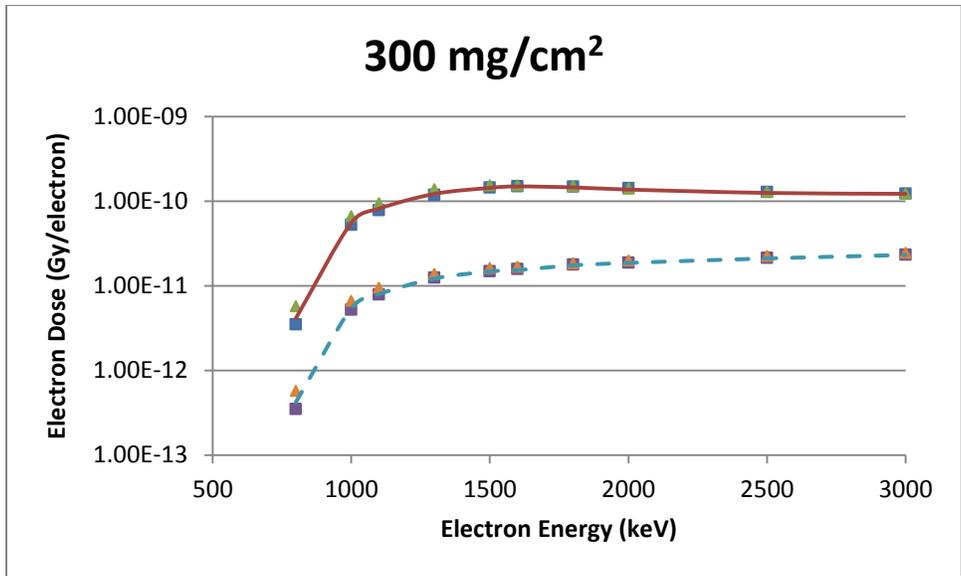
**Figure B-3** A Point Source Geometry Comparison of VARSKIN 5 (boxes), MCNP5 (triangles) and EGSnrc (lines) Predicted Dose Per Initial Electron as a Function of Electron Energy in Tissue at a Density Thickness of 300 mg/cm<sup>2</sup> and a 20 mm Thick Tissue Volume Cylinder of Area 1 cm<sup>2</sup> (solid line) and 10 cm<sup>2</sup> (dashed line)
