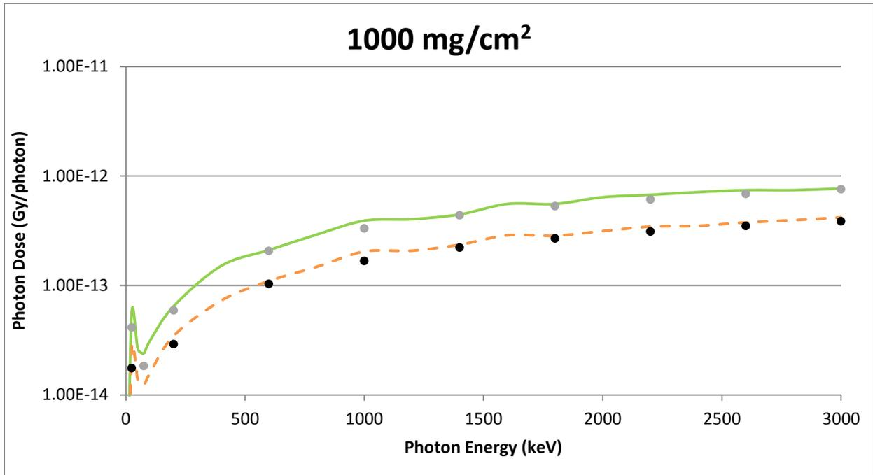
**Figure A-4** A Point Source Geometry Comparison of VARSKIN 5 (circles) and MCNP5 (lines) Predicted Dose Per Initial Photon as a Function of Photon Energy in Tissue at a Density Thickness of 1000 mg/cm<sup>2</sup> and a Tissue Volume Cylinder of Area 1 cm<sup>2</sup> (solid line) and 10 cm<sup>2</sup> (dashed line), With a Thickness of 20 mm
