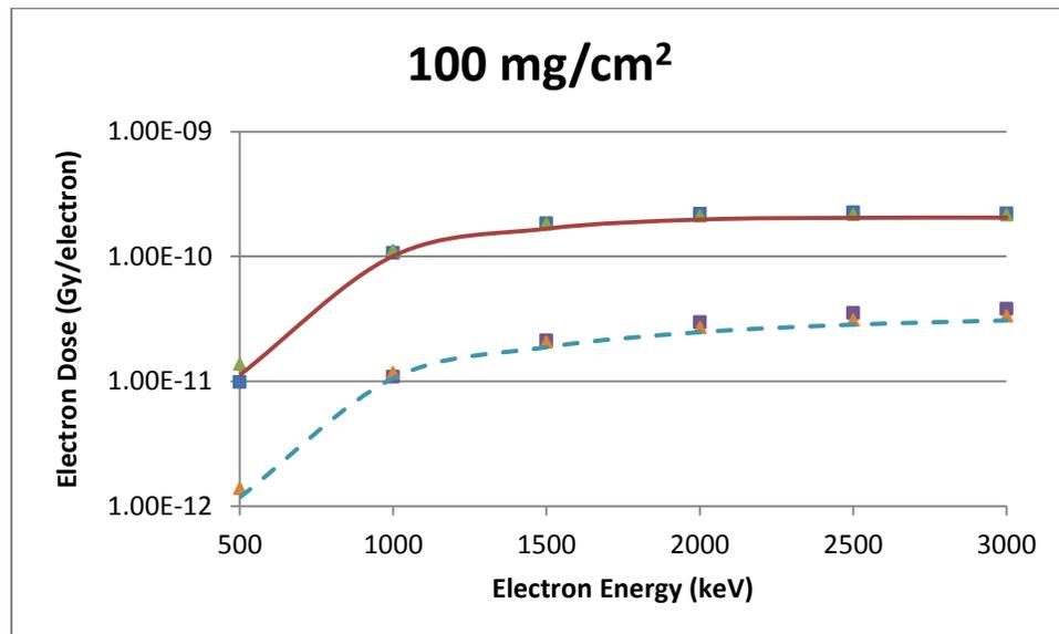
Figure B-34 A Cylindrical Source Geometry Comparison of VARSKIN 5 (boxes), MCNP5 (triangles) and EGSnrc (lines) Predicted Dose Per Initial Electron as a Function of Electron Energy in Tissue at a Density Thickness of 100 mg/cm<sup>2</sup> and a Tissue Volume Cylinder of Area 1 cm<sup>2</sup> (solid line) and 10 cm<sup>2</sup> (dashed line), With a Thickness of 20 mm
