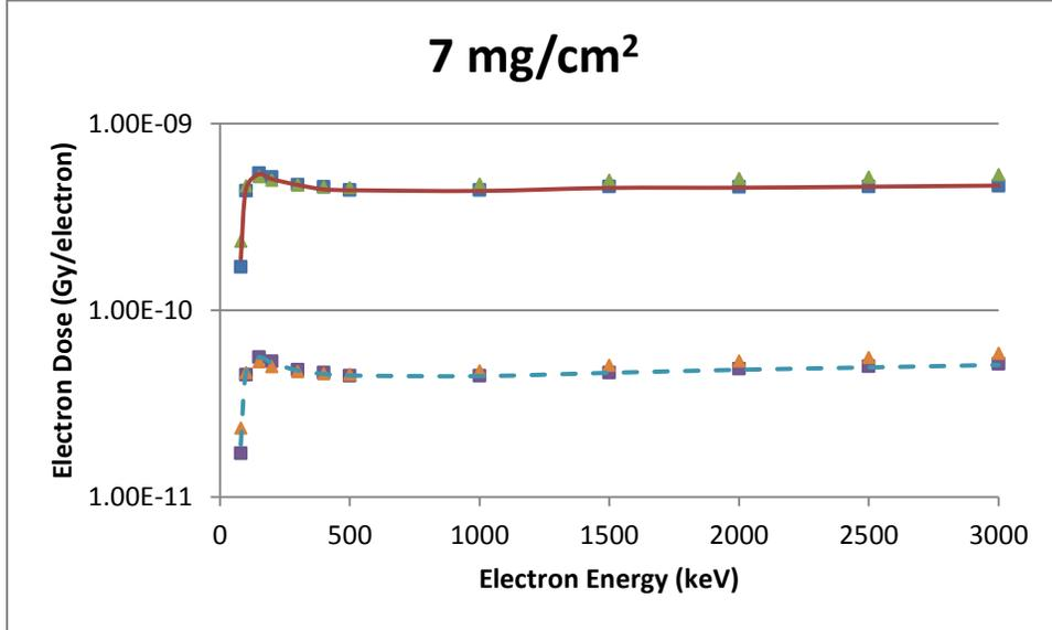
**Figure B-1** A Point Source Geometry Comparison of VARSKIN 5 (boxes), MCNP5 (triangles) and EGSnrc (lines) Predicted Dose Per Initial Electron as a Function of Electron Energy in Tissue at a Density Thickness of 7 mg/cm<sup>2</sup> and a 20 mm Thick Tissue Volume Cylinder of Area 1 cm<sup>2</sup> (solid line) and 10 cm<sup>2</sup> (dashed line)
