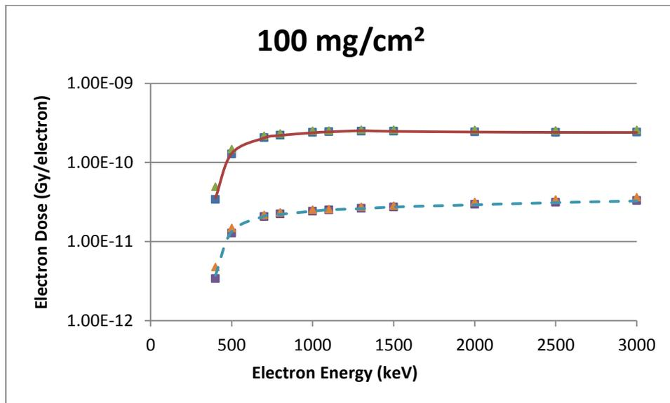
Figure B-26 A 5 mm Diameter Disk Source Geometry Comparison of VARSKIN 5 (boxes), MCNP5 (triangles) and EGSnrc (lines) Predicted Dose Per Initial Electron as a Function of Electron Energy in Tissue at a Density Thickness of 100 mg/cm<sup>2</sup> and a Tissue Volume Cylinder of Area 1 cm<sup>2</sup> (solid line) and 10 cm<sup>2</sup> (dashed line), With a Thickness of 20 mm
