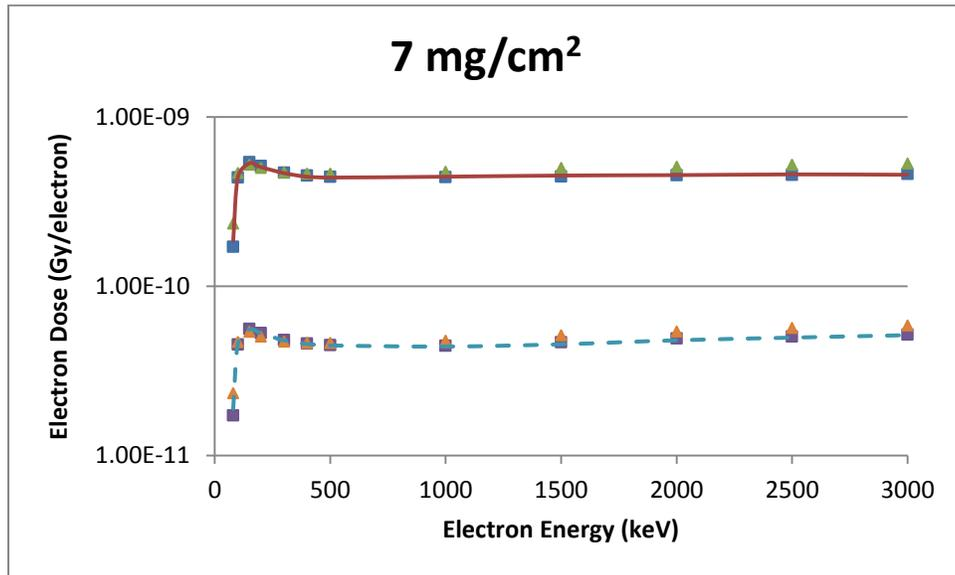
Figure B-25 A 5 mm Diameter Disk Source Geometry Comparison of VARSKIN 5 (boxes), MCNP5 (triangles) And EGSnrc (lines) Predicted Dose Per Initial Electron as a Function of Electron Energy in Tissue at a Density Thickness of 7 mg/cm<sup>2</sup> and a Tissue Volume Cylinder of Area 1 cm<sup>2</sup> (solid line) and 10 cm<sup>2</sup> (dashed line), With a Thickness of 20 mm
