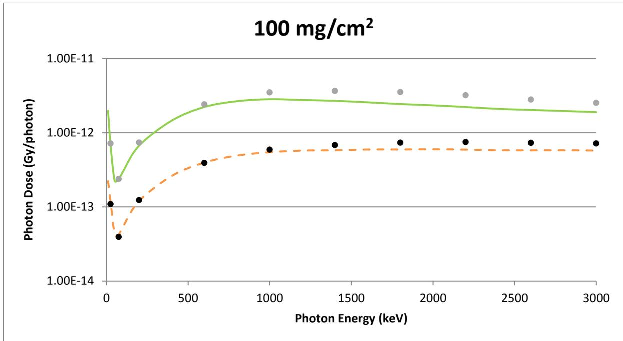
**Figure A-10** A Cylindrical Source Geometry Comparison of VARSKIN 5 (circles) and MCNP5 (lines) Predicted Dose Per Initial Photon as a Function of Photon Energy in Tissue at a Density Thickness of 100 mg/cm<sup>2</sup> and a Tissue Volume Cylinder of Area 1 cm<sup>2</sup> (solid line) and 10 cm<sup>2</sup> (dashed line), With a Thickness of 20 mm
