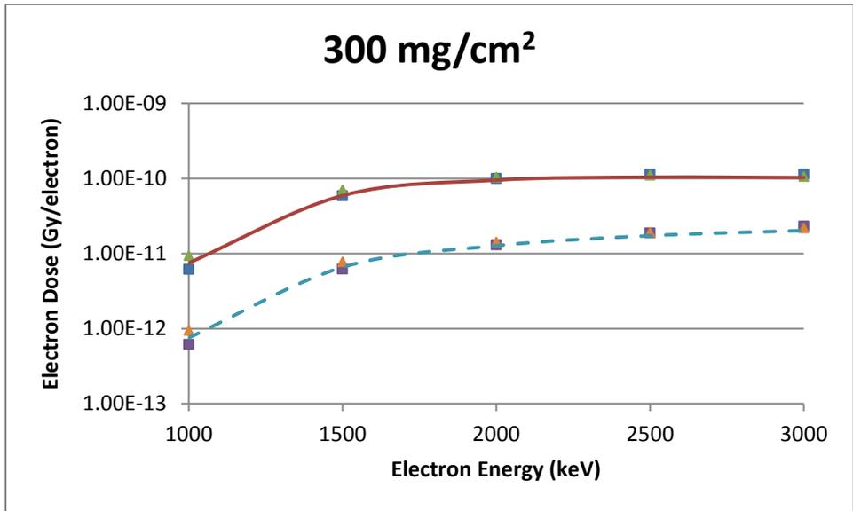
**Figure B-35** A Cylindrical Source Geometry Comparison of VARSKIN 5 (boxes), MCNP5 (triangles) and EGSnrc (lines) Predicted Dose Per Initial Electron as a Function of Electron Energy in Tissue at a Density Thickness of 300 mg/cm<sup>2</sup> and a Tissue Volume Cylinder of Area 1 cm<sup>2</sup> (solid line) and 10 cm<sup>2</sup> (dashed line), With a Thickness of 20 mm
