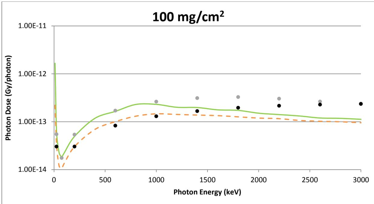
**Figure A-22 A Point Source Geometry With a Cotton Cover and a 1 cm Air Gap Comparison of VARSKIN 5 (circles) and MCNP5 (lines) Predicted Dose Per Initial Photon as a Function of Photon Energy in Tissue at a Density Thickness of 100 mg/cm<sup>2</sup> and a Tissue Volume Cylinder of Area 1 cm<sup>2</sup> (solid line) and 10 cm<sup>2</sup> (dashed line); Thickness of 20 mm**
