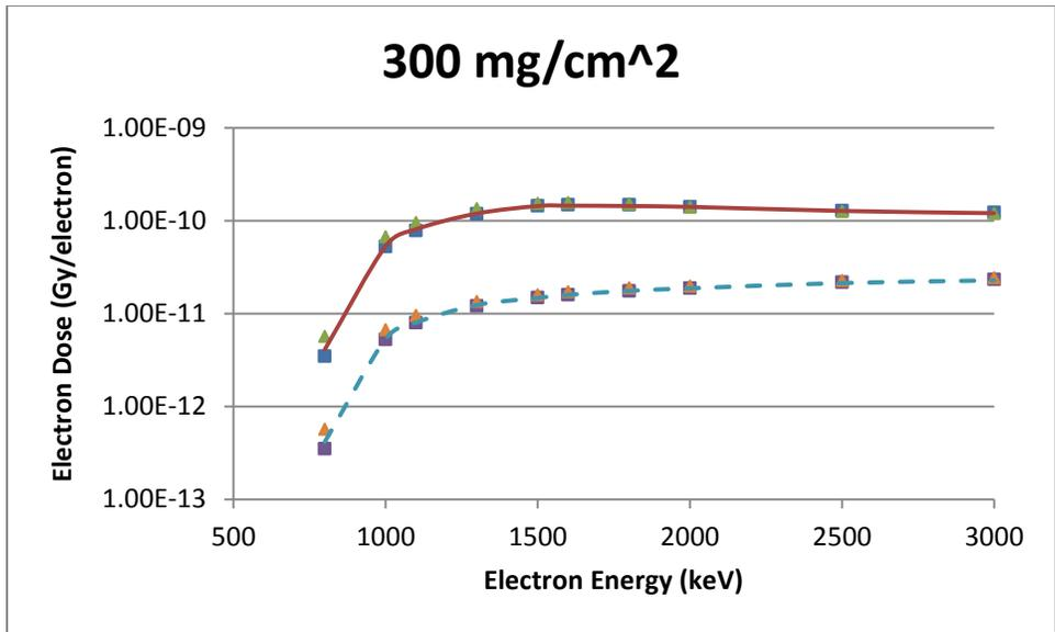
**Figure B-19** A 1 mm Diameter Disk Source Geometry Comparison of VARSKIN 5 (boxes), MCNP5 (triangles) and EGSnrc (lines) Predicted Dose Per Initial Electron as a Function of Electron Energy in Tissue at a Density Thickness of 300 mg/cm<sup>2</sup> and a Tissue Volume Cylinder of Area 1 cm<sup>2</sup> (solid line) and 10 cm<sup>2</sup> (dashed line), With a Thickness of 20 mm
