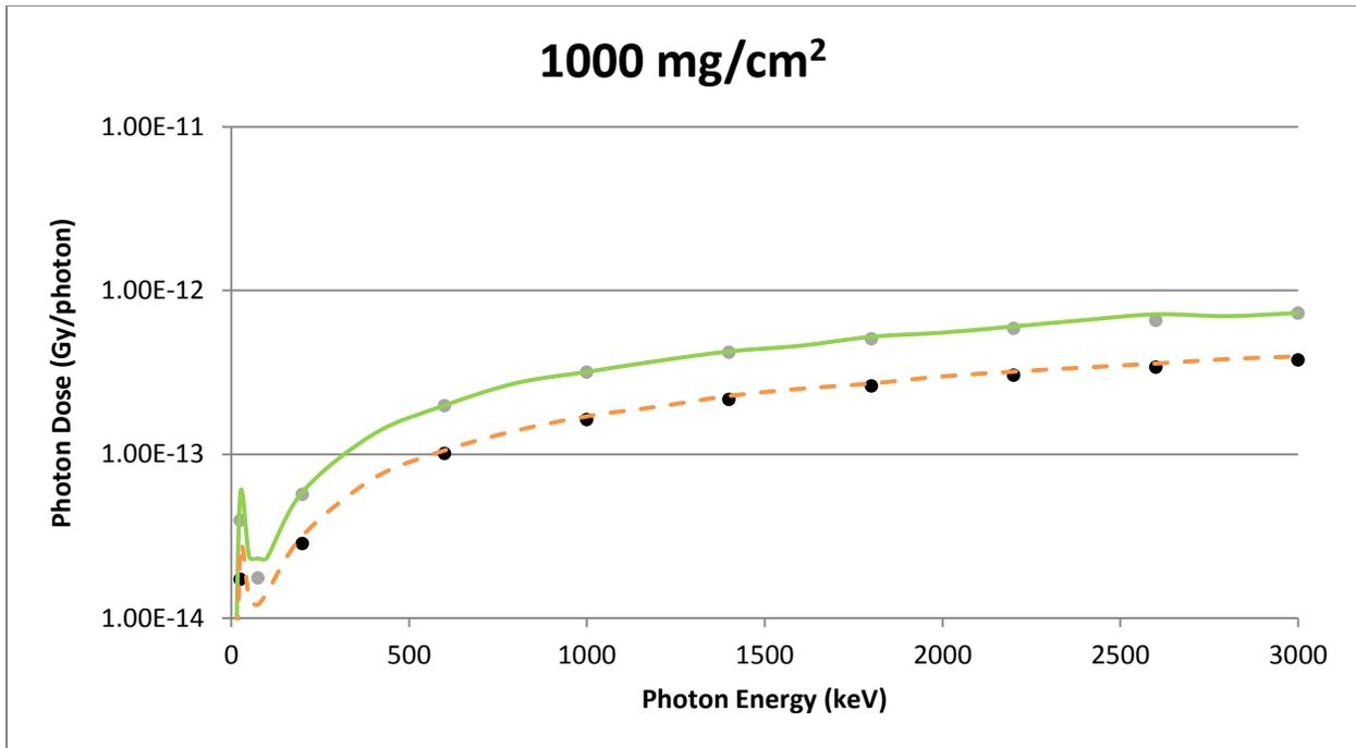
**Figure A-12** A Cylindrical Source Geometry Comparison of VARSKIN 5 (circles) and MCNP5 (lines) Predicted Dose Per Initial Photon as a Function of Photon Energy In Tissue at a Density Thickness of 1000 mg/cm<sup>2</sup> and a Tissue Volume Cylinder of Area 1 cm<sup>2</sup> (solid line) and 10 cm<sup>2</sup> (dashed line), With a Thickness of 20 mm
