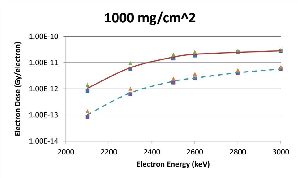
**Figure B-20** A 1 mm Diameter Disk Source Geometry Comparison of VARSKIN 5 (boxes), MCNP5 (triangles) and EGSnrc (lines) Predicted Dose Per Initial Electron as a Function of Electron Energy in Tissue at a Density Thickness of 1000 mg/cm<sup>2</sup> and a Tissue Volume Cylinder of Area 1 cm<sup>2</sup> (solid line) and 10 cm<sup>2</sup> (dashed line), With a Thickness of 20 mm
