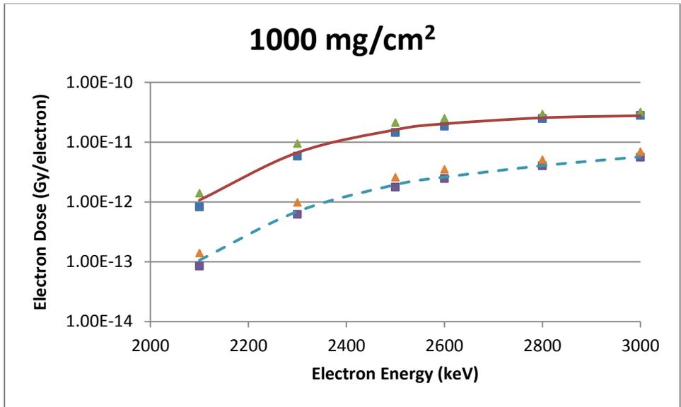
**Figure B-4** A Point Source Geometry Comparison of VARSKIN 5 (boxes), MCNP5 (triangles) and EGSnrc (lines) Predicted Dose Per Initial Electron as a Function of Electron Energy in Tissue at a Density Thickness of 1000 mg/cm<sup>2</sup> and a 20 mm Thick Tissue Volume Cylinder of Area 1 cm<sup>2</sup> (solid line) and 10 cm<sup>2</sup> (dashed line)
