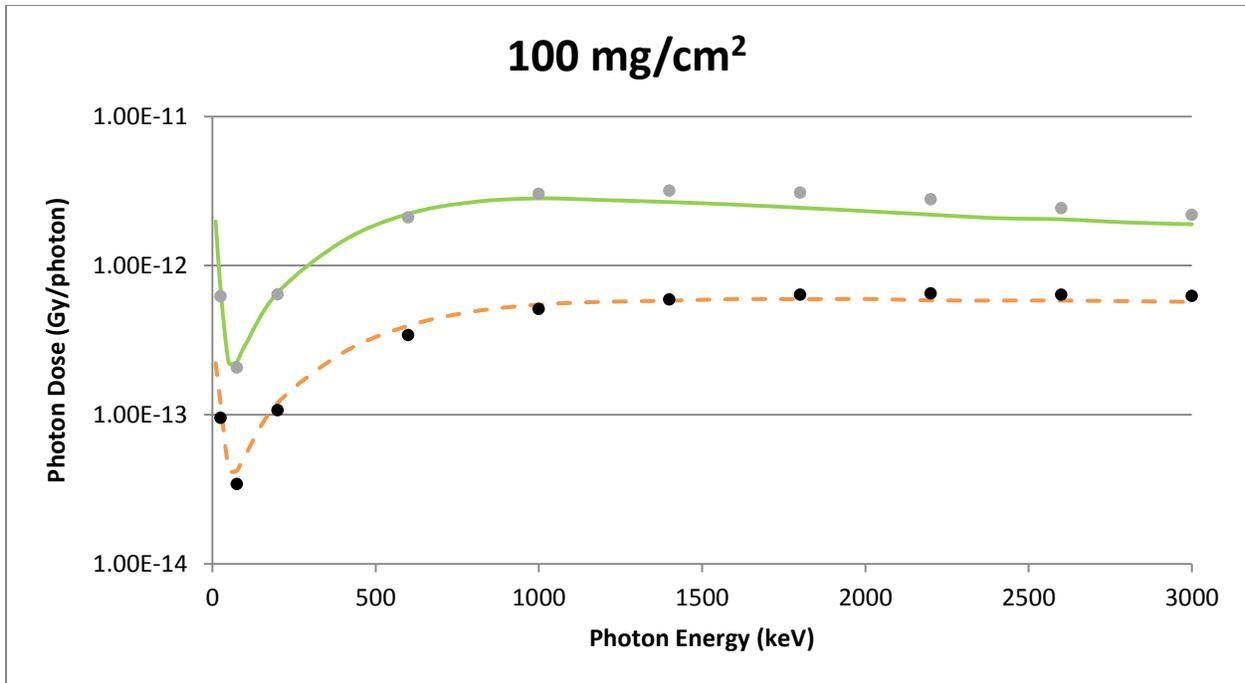
**Figure A-14** A Slab Source Geometry Comparison of VARSKIN 5 (circles) and MCNP5 (lines) Predicted Dose Per Initial Photon as a Function of Photon Energy in Tissue at a Density Thickness of 100 mg/cm<sup>2</sup> and a Tissue Volume Cylinder of Area 1 cm<sup>2</sup> (solid line) and 10 cm<sup>2</sup> (dashed line), With a Thickness of 20 mm
