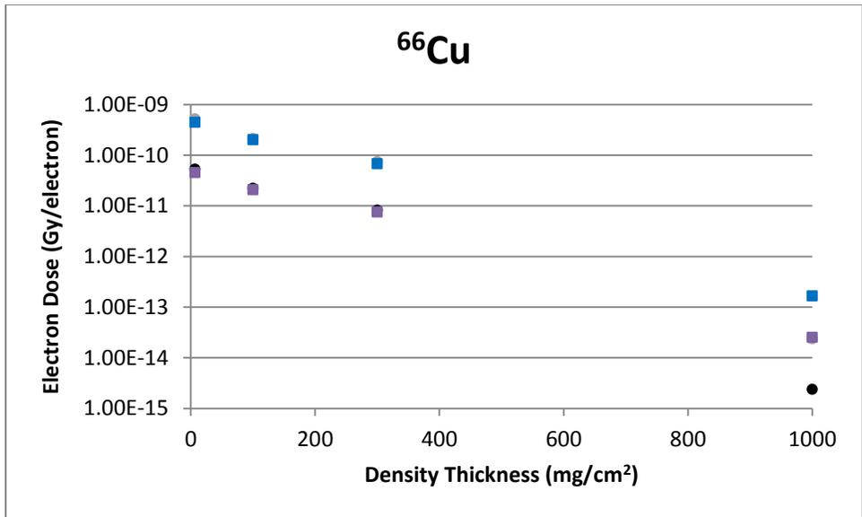
**Figure B-7** A Point Source Geometry Comparison of VARSKIN 5 (boxes) and VARSKIN 4 (circles) Predicted Dose Per Initial Beta From  $^{66}\text{Cu}$  as a Function of Density Thickness in Tissue and a Tissue Volume Cylinder of Area 1 cm<sup>2</sup> (upper) and 10 cm<sup>2</sup> (lower), With a Thickness of 20 mm
