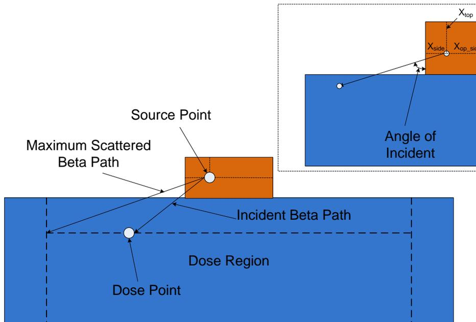
**Figure 3-9 Schematic Illustrating Parameters Used for Side Scattering**
