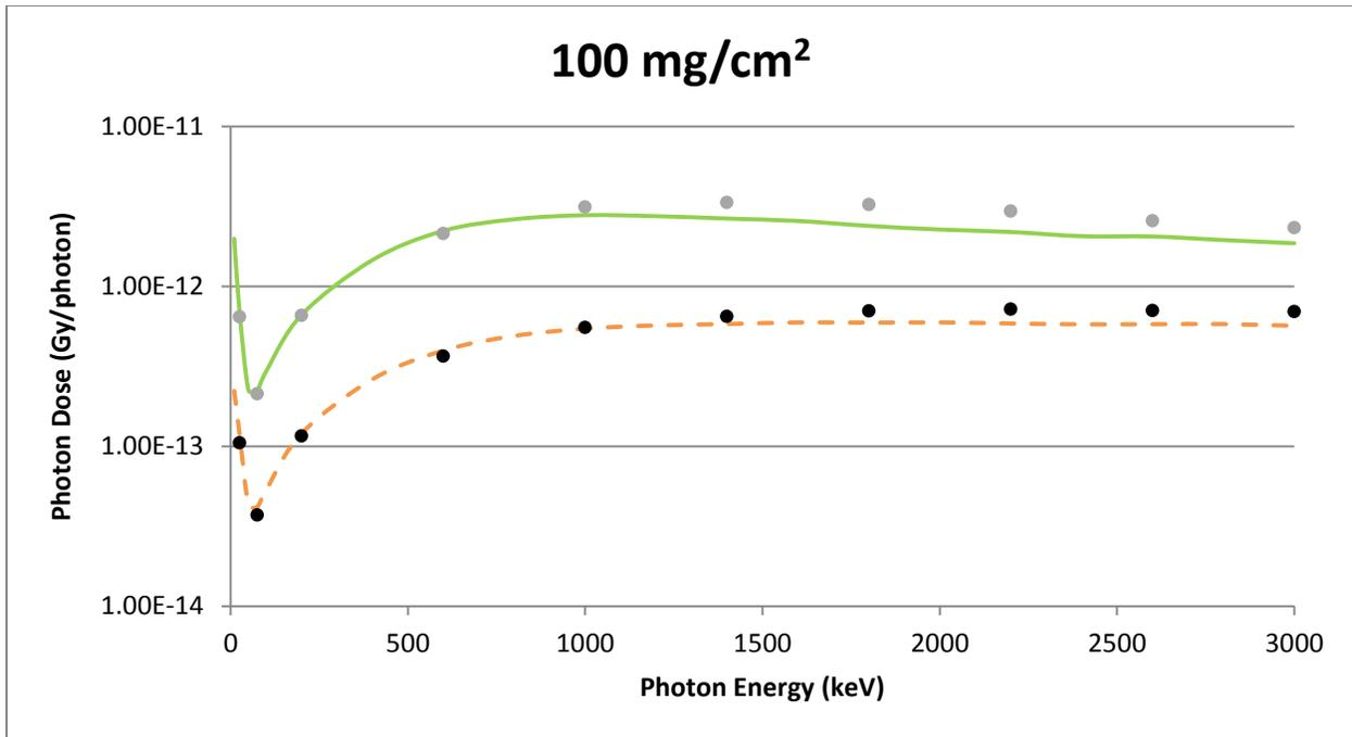
**Figure A-18 A Spherical Source Geometry Comparison of VARSKIN 5 (circles) and MCNP5 (lines) Predicted Dose Per Initial Photon as a Function of Photon Energy in Tissue at a Density Thickness of 100 mg/cm<sup>2</sup> and a Tissue Volume Cylinder of Area 1 cm<sup>2</sup> (solid line) and 10 cm<sup>2</sup> (dashed line), With a thickness of 20 mm**
