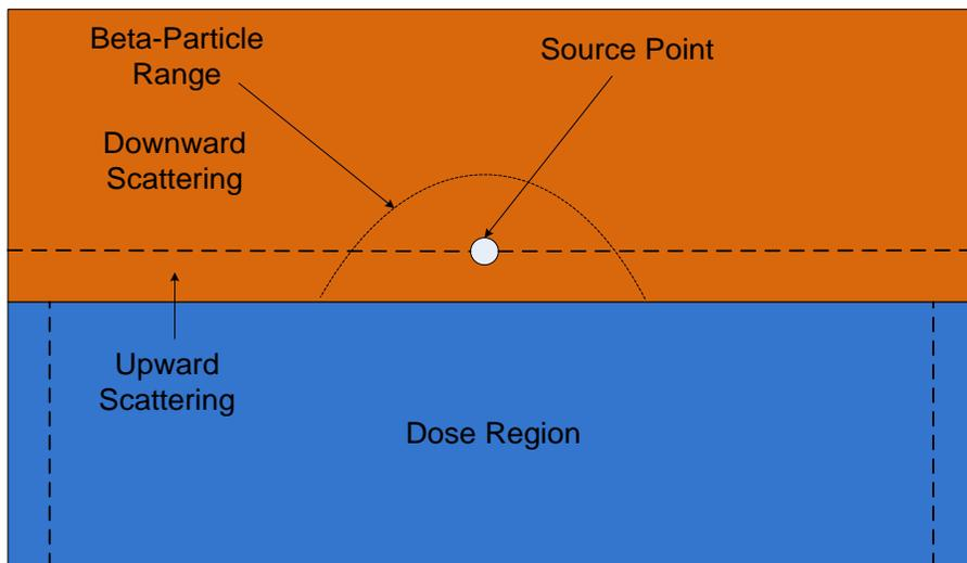
**Figure 3-7 Schematic Demonstrating Conditions for Partial Source Scattering Conditions**
