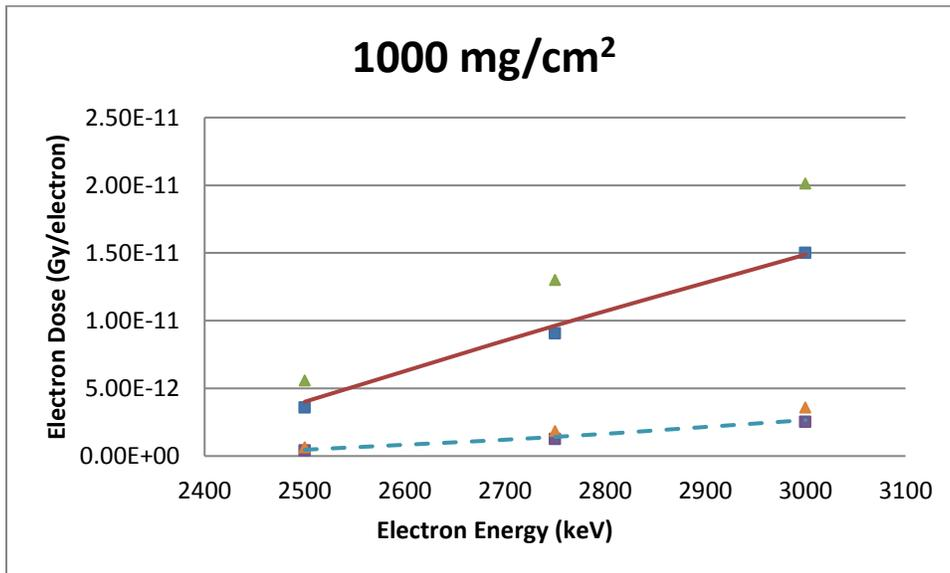
**Figure B-44** A Spherical Source Geometry Comparison of VARSKIN 5 (boxes), MCNP5 (triangles) and EGSnrc (lines) Predicted Dose Per Initial Electron as a Function of Electron Energy in Tissue at a Density Thickness of 1000 mg/cm<sup>2</sup> and a Tissue Volume Cylinder of Area 1 cm<sup>2</sup> (solid line) and 10 cm<sup>2</sup> (dashed line), With a Thickness of 20 mm
