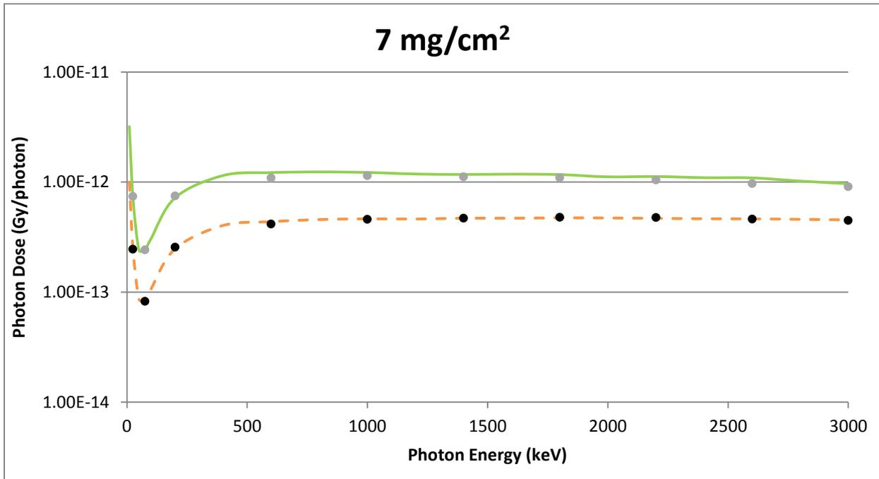
**Figure A-5** A Disk Source Geometry Comparison of VARSKIN 5 (circles) and MCNP5 (lines) Predicted Dose Per Initial Photon as a Function of Photon Energy in Tissue at a Density Thickness of 7 mg/cm<sup>2</sup> and a Tissue Volume Cylinder of Area 1 cm<sup>2</sup> (solid line) and 10 cm<sup>2</sup> (dashed line), With a Thickness of 20 mm
