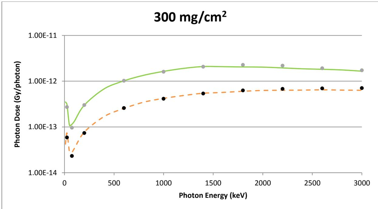
**Figure A-19 A Spherical Source Geometry Comparison of VARSKIN 5 (circles) and MCNP5 (lines) Predicted Dose Per Initial Photon as a Function of Photon Energy in Tissue at a Density Thickness of 300 mg/cm<sup>2</sup> and a Tissue Volume Cylinder of Area 1 cm<sup>2</sup> (solid line) and 10 cm<sup>2</sup> (dashed line), With a Thickness of 20 mm**
