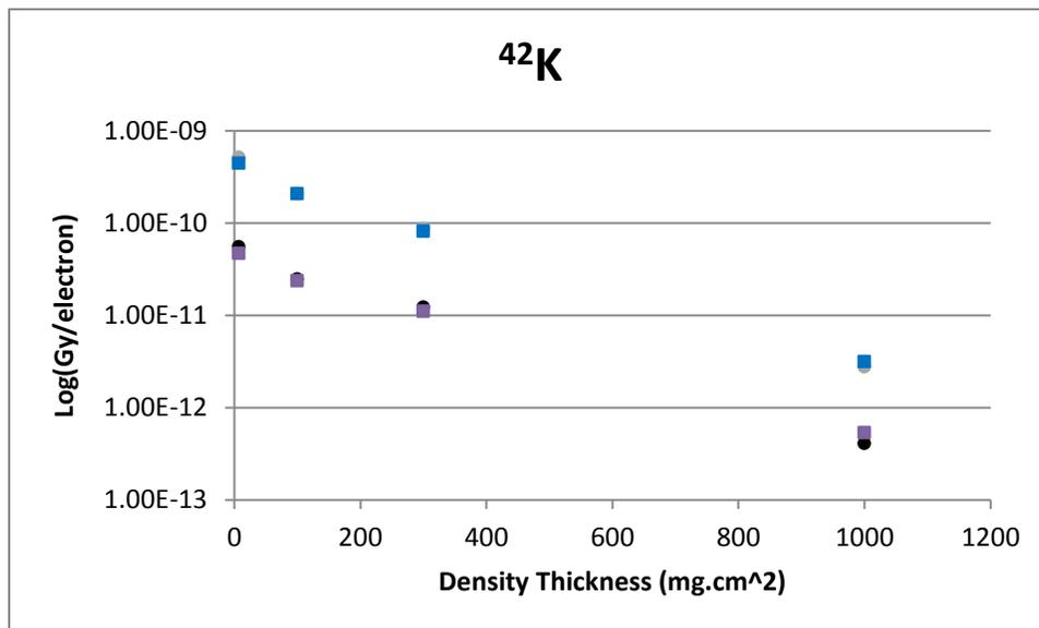
**Figure B-30** A 5 mm Diameter Disk Geometry Comparison of VARSKIN 5 (boxes) and VARSKIN 4 (circles) Predicted Dose Per Initial Beta From  $^{42}\text{K}$  as a Function of Density Thickness in Tissue and a Tissue Volume Cylinder of Area 1 cm<sup>2</sup> (upper) and 10 cm<sup>2</sup> (lower), With a Thickness of 20 mm
