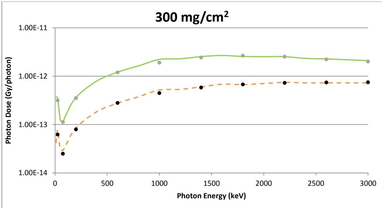
**Figure A-3** A Point Source Geometry Comparison of VARSKIN 5 (circles) and MCNP5 (lines) Predicted Dose Per Initial Photon as a Function of Photon Energy in Tissue at a Density Thickness of 300 mg/cm<sup>2</sup> and a Tissue Volume Cylinder of Area 1 cm<sup>2</sup> (solid line) and 10 cm<sup>2</sup> (dashed line), With a Thickness of 20 mm
