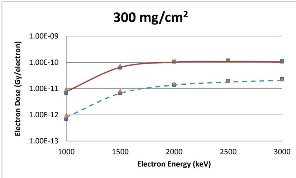
**Figure B-43** A Spherical Source Geometry Comparison of VARSKIN 5 (boxes), MCNP5 (triangles) and EGSnrc (lines) Predicted Dose Per Initial Electron as a Function of Electron Energy in Tissue at a Density Thickness of 300 mg/cm<sup>2</sup> and a Tissue Volume Cylinder of Area 1 cm<sup>2</sup> (solid line) and 10 cm<sup>2</sup> (dashed line), With a Thickness of 20 mm
