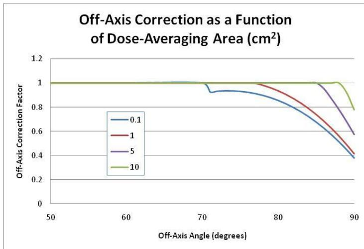
**Figure 3-19 Off-Axis Correction Factor as a Function of Off-Axis Angle and Dose-Averaging Area**
