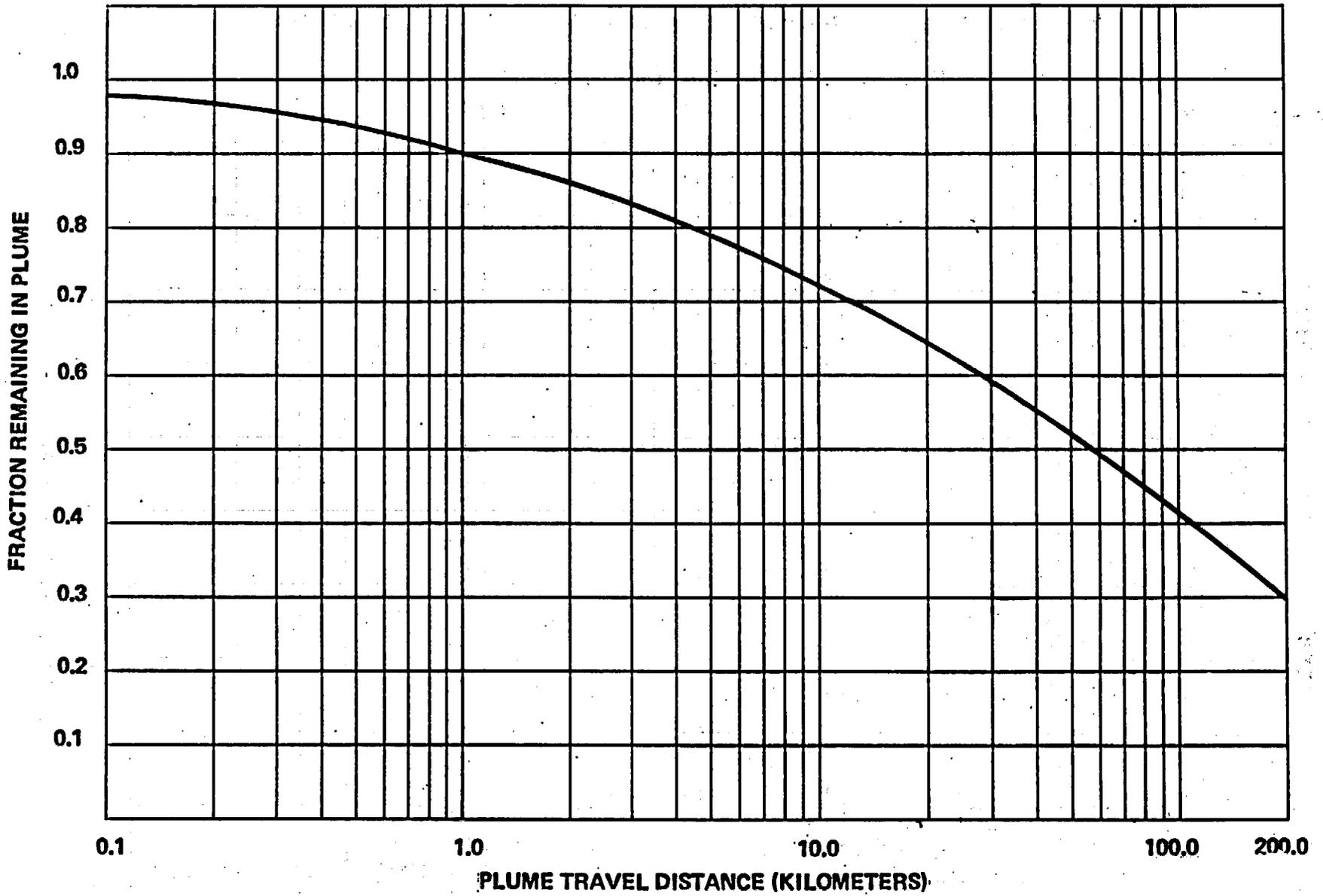
Figure 2. Plume Depletion Effect for Ground-Level Releases (All Atmospheric Stability Classes)
