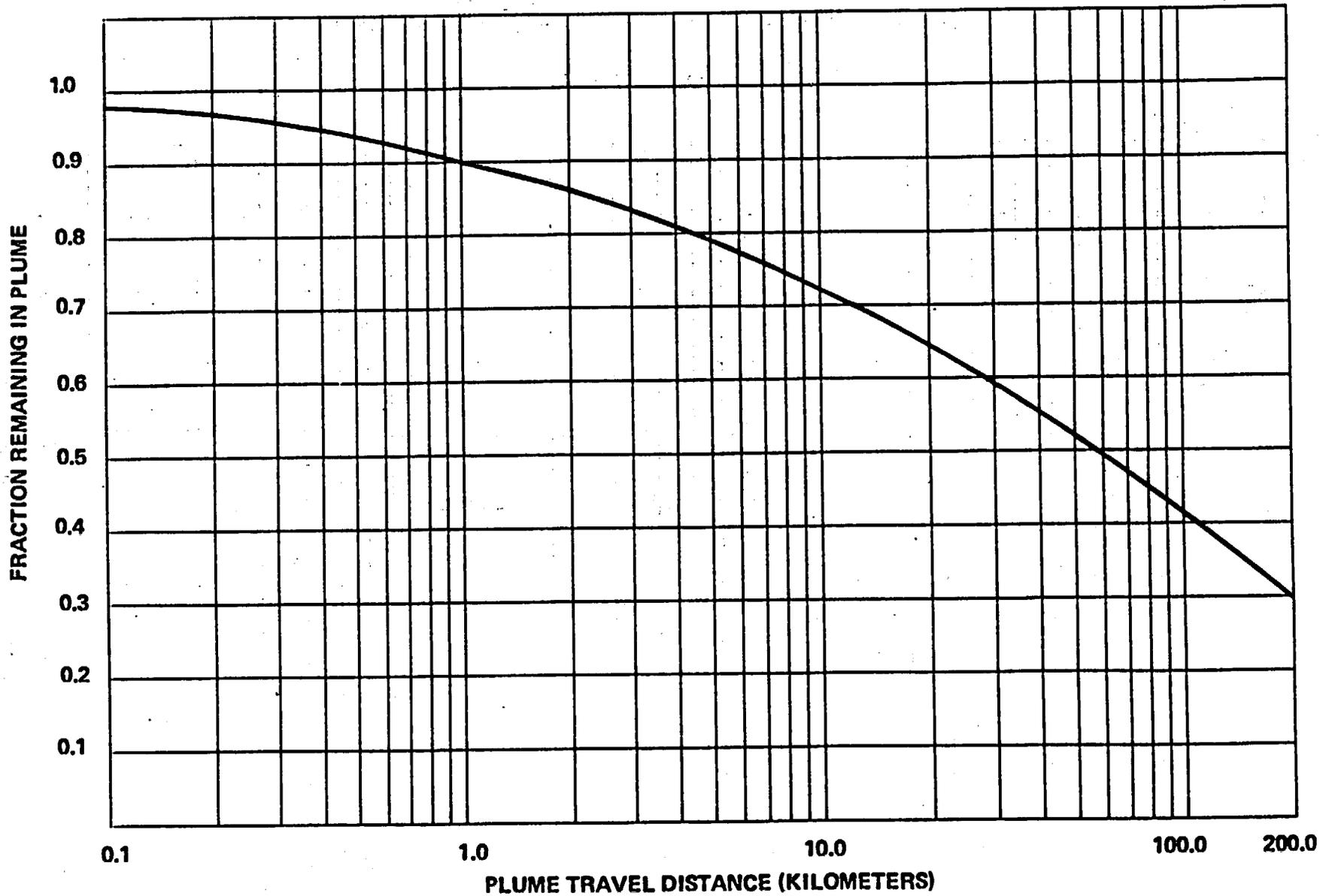
Figure 3. Plume Depletion Effect for Ground Level Releases (All Atmospheric Stability Classes)
