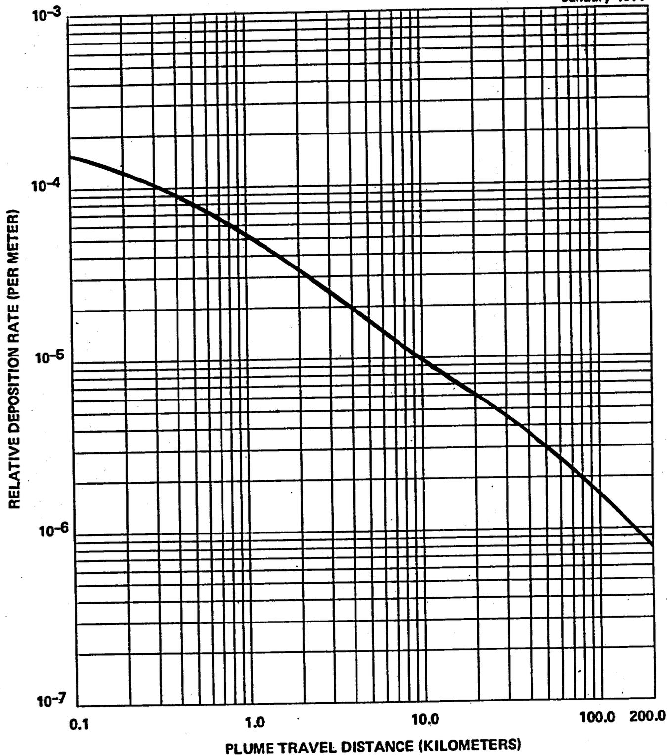
Figure 7. Relative Deposition for Ground Level Releases (All Atmospheric Stability Classes)
