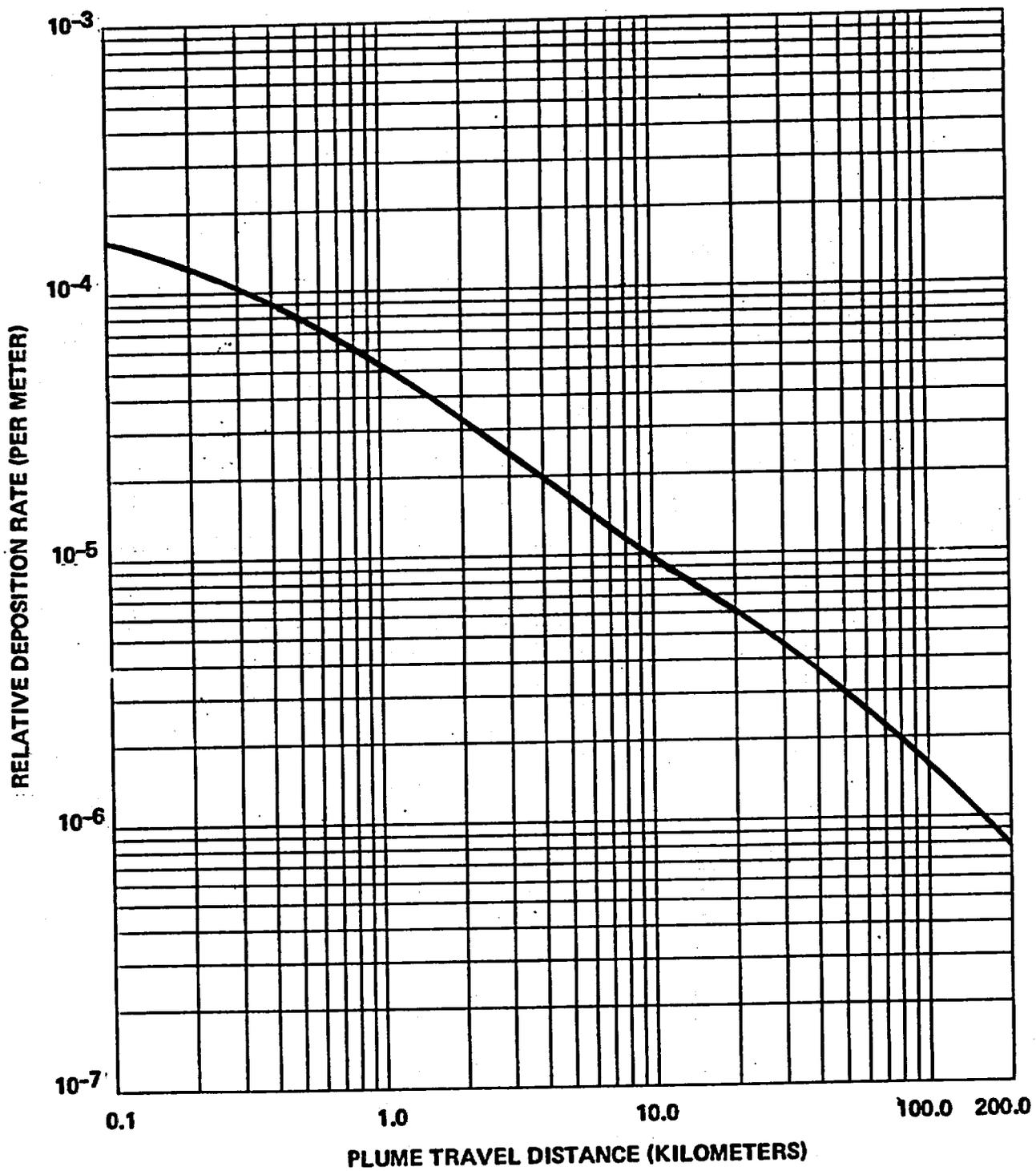
Figure 6. Relative Deposition for Ground-Level Releases (All Atmospheric Stability Classes)
