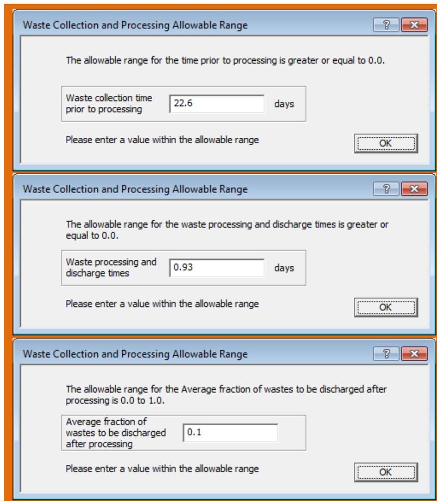
**Figure 3-26 Waste Collection and Processing Allowable Range Screens**
