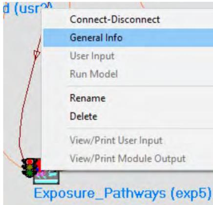
The following window Object General Information opens. Notice in this example the Northing coordinate is 10 km. *GENII will take the nearest grid point to this location and make calculations at only this location.*
