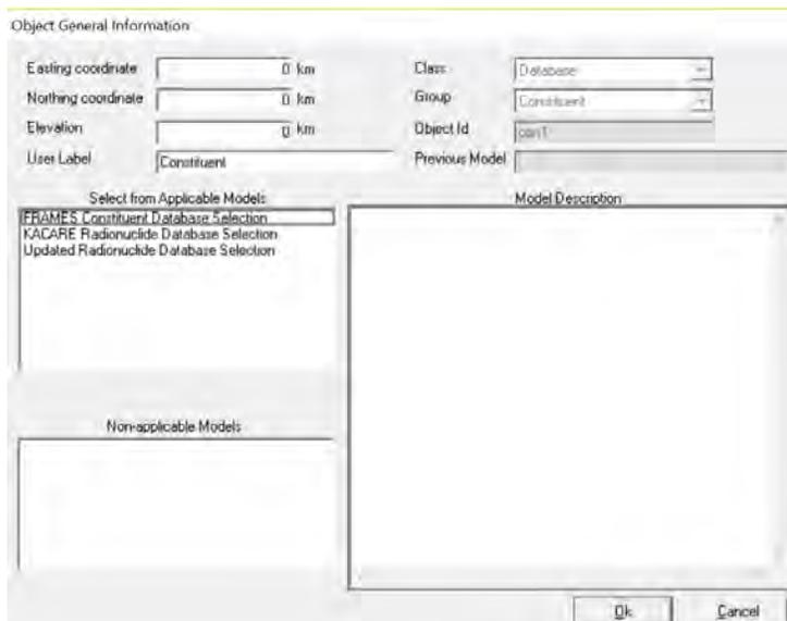
Under Select from Applicable Models three options are provided: FRAMES Constituent Database Selection, KACARE Radionuclide Database Selection, and Updated Radionuclide Database Selection. Select the third model: Updated Radionuclide Database Selection. The Model Description is shown in the window to the right. Select Ok.
