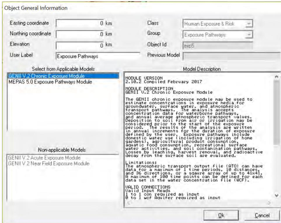
Select Ok; the Object General Information window closes, and the icon Exposure Pathways (exp4) now shows a red light in the “traffic signal”. *Note that the Northing and Easting are both zero – this is a signal to the model to use **all** locations on the atmospheric dispersion grid.*
