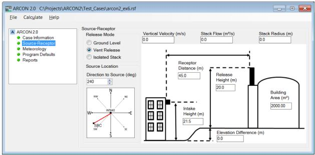
Figure 4-16. ARCON 2.0 Source-Receptor Form for Example 6
