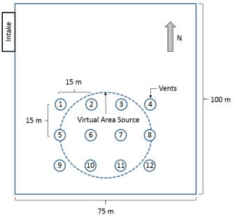
Figure 4-11 Multiple-vent release configuration for Example 5
