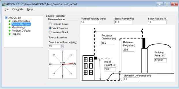
Figure 4-4 ARCON 2.0 Source-Receptor Form for Example 2
