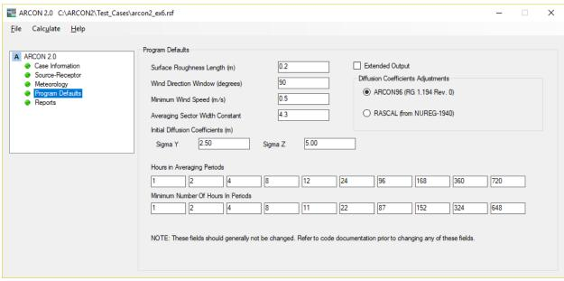
Figure 4-17 ARCON 2.0 Program Defaults Form for Example 6
