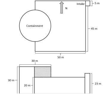
Figure 4-15. Diffuse-source release configuration for Example 6
