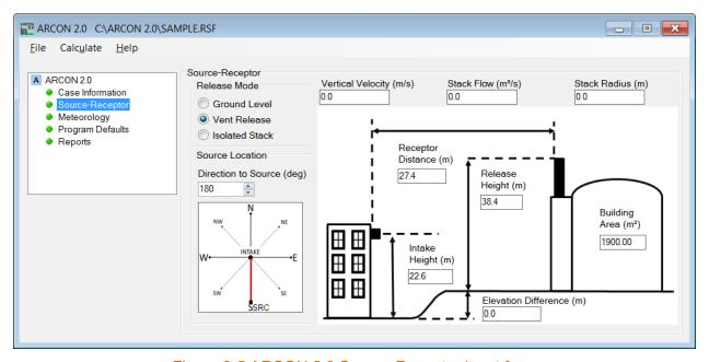
Figure 2-5 ARCON 2.0 Source-Receptor input form
