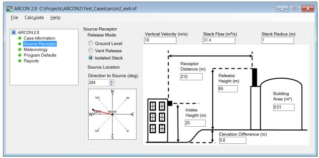
Figure 4-8 ARCON 2.0 Source-Receptor Form for Example 4
