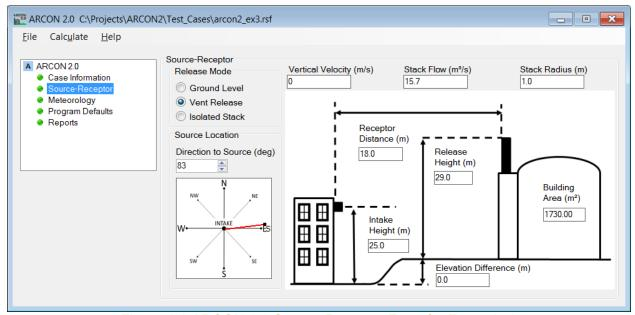
Figure 4-6 ARCON 2.0 Source-Receptor Form for Example 3
