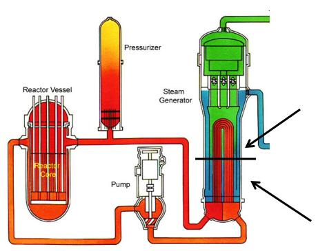
Leak above the water – most nuclides available for release; 50% of non-nobles escape.
