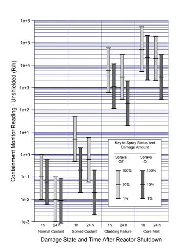
The model uses tables such as this one to convert the reading into a damage amount.
