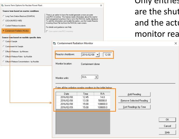
Only entries required are the shutdown time and the actual rad monitor readings.
