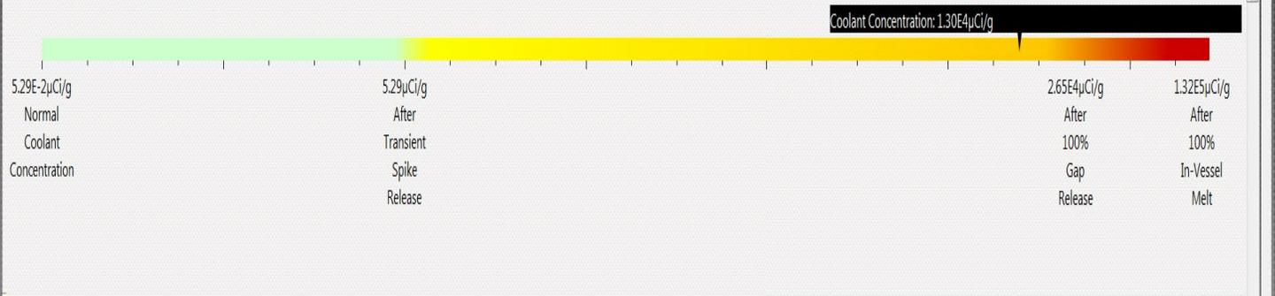
⚠ The Coolant Concentration level indicates that Gap Releases have occurred and Fuel Melt may have initiated.
